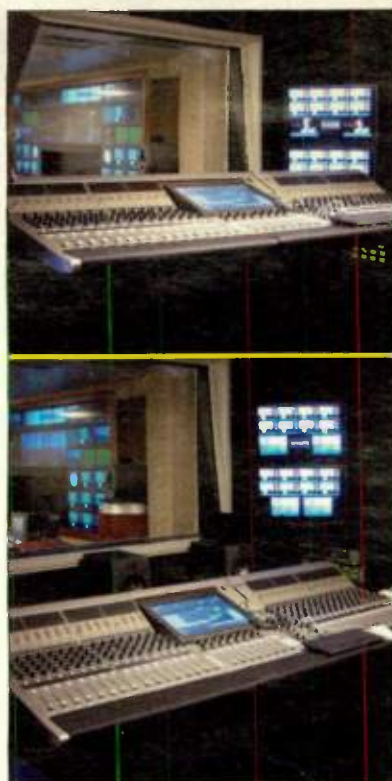
Now it's up, now it's down—the Newseum's Euphonix audio consoles ride on an elevator to adapt to operator requirements.
