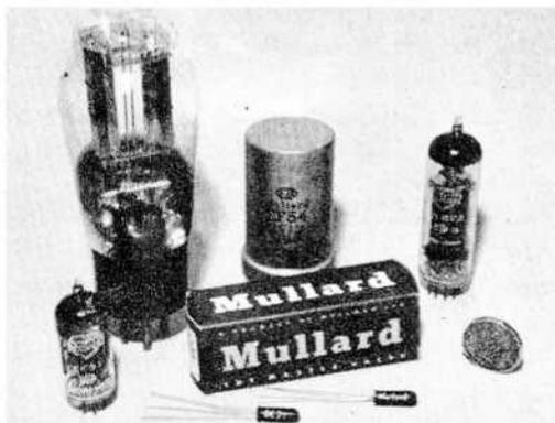
● A group of typical radio valves. Left to right: miniature h.f. pentode, h.t. rectifier, earlier type of h.f. pentode in metal case, output valve (miniature type). Compare the size of the valves with the two transistors at the foot of the picture.
