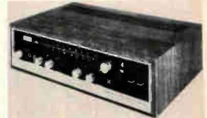
amic power into 4 ohms. Harmonic distortion for this amplifier is said to be less than 0.8% at rated output and frequency response is 30-30,000 Hz at  $\pm 1.0$  dB. Otherwise, specifications of the *Models QR-500* and *QR-1500* are identical.
