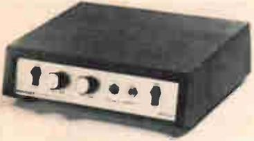
tuner input, both channels driven); THD speakers less than 2%, phones less than 0.5%; max. sine-wave output speakers & phones 500 mW into 8 ohms both channels driven; hum level 75 dB below full output on mag. phono inputs; front-panel input (tuner-phonon) selector; left & right vol; two parallel stereo headphone jacks; illuminated power switch; rear-panel mag. phono input; tuner input; speaker output; speaker-phones switch; over-all size 3" x 10 1/2" x 8 1/2" D; \$79.95.
