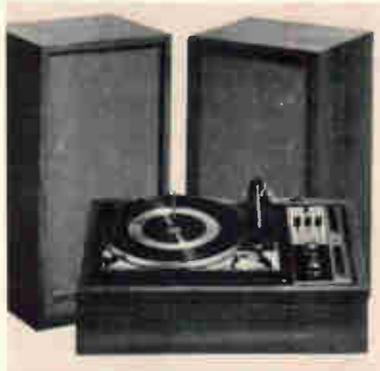
diamond stylus; 20 W/channel continuous sine-wave (into 8 ohms) power amp, both channels driven; AM-FM tuner section; pair of KLH speaker systems; features tape monitoring & recording facilities; outputs for remote & main speakers; speaker cabinets 23 1/2" x 12 3/8" x 11 7/8" D; 12" acoustic-suspension woofer; 1 3/4" direct-radiator tweeter; 1500 Hz LCR crossover; control center 9" x 20 1/2" x 14 3/8" D; oiled walnut finish; \$549.95
