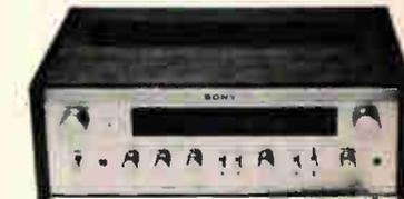
has virtually the same list of features as the 6065, including similar direct-coupled circuitry. Power is a hefty 145 watts IHF into 4 ohms (100 watts IHF into 8 ohms) 40/40 watts continuous at 8 ohms. IHF FM sensitivity is a notable 2.6 uV; selectivity and capture ratio are 80 dB and 1.5 dB respectively.
