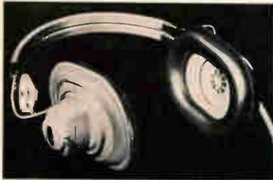
1000 Hz produces 112 dB SPL; distortion <1% at 125 dB SPL; 600 ohms impedance; weight 11 oz; \$39.50.
