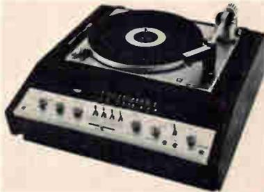
mag. cartridge; diamond stylus; Dustamatic brush; 35 W/channel continuous sine-wave into 8 ohms with both channels driven at 0.5% THD; 57 W/channel dynamic power at 8 ohms; 75 W/channel into 4 ohms; power bandwidth 18-30,000 Hz; response 13-70,000 Hz ±1.5 dB; AM-Stereo FM tuner section with 1.8 μV FM sensitivity for 30 dB quieting; capture ratio 2.5 dB (IHF); main/remote speaker switch; control center 17 1/4" x 8" x 18" D; without speakers; oiled walnut cabinet; \$349.95
