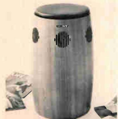
motifs; response 50-18,000 Hz (reference not stated); 8 ohms impedance; 50 watts (IHF) maximum input power; 24" H x 16" diameter; oiled walnut; foam-filled top cushion; weight 30 lbs; \$149.50.
