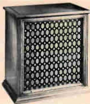
standing with 15" woofer and Sectoral horn mid-range/tweeter; response 30-20,000 Hz (reference not stated); 80 Hz crossover frequency; horn level control; 8 ohms impedance; 50 watts (rms) maximum input power; 29 $\frac{3}{8}$ " H x 27 $\frac{3}{4}$ " W x 19 $\frac{3}{8}$ " D; similar to Altec "Milano"; \$259.95 (kit).
