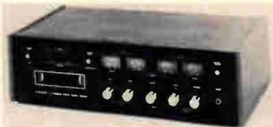
built-in 8-track, 4- or 2-channel compatible cartridge tape playback system. The power output rating of the *Model 702* is 20 W rms (total). Trademarked a "Qaudio" system, the *Model 702* has four independent VU meters, ganged tone controls and a loudness compensation switch. The manufacturer claims a frequency response of 100-10,000 Hz and wow & flutter at 3000 Hz of 0.35%. The *Model 702* measures 5 $\frac{1}{2}$ " H x 18 $\frac{3}{4}$ " W x 10" D.
