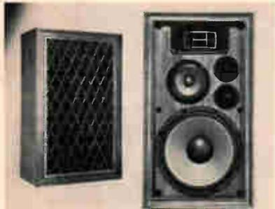
tweeter; response 35-20,000 Hz (reference not stated); 500 Hz and 4500 Hz crossover frequencies; mid-range and tweeter controls on front panel; 8 ohms impedance; 60 watts (dynamic) maximum input power; 26" H x 12 3/4" W x 15" D; walnut; individual speaker connections to manufacturer's multi-amp system; weight 37 lbs; \$189.00.
