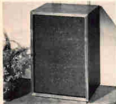
range, and horn-type tweeter; response 70-17,000 Hz at ±5 dB (reference not stated); 700 Hz and 6000 Hz crossover frequencies; 16 ohms impedance; 25 watts (dynamic) maximum input power; 21<sup>3</sup>/<sub>8</sub>" H x 15<sup>1</sup>/<sub>2</sub>" W x 13<sup>1</sup>/<sub>8</sub>" D; furniture finishes; weight 55 lbs; \$252.00.
