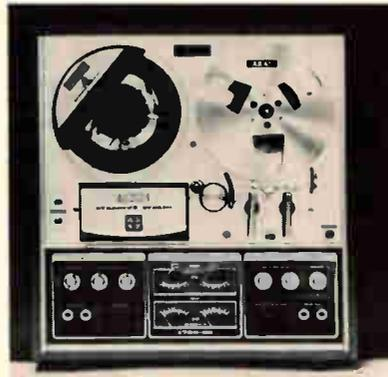
with a frequency response of 30-22,000 Hz at  $\pm 3.0$  dB. The wow & flutter (also measured at 7½ ips) is claimed by the manufacturer to be 0.12% rms. The *Model 1730D-SS* has four heads—one each for recording and playback and two erase heads (2-channel and full-track). There are four independent VU meters, fully automatic shut-off, headphone jacks for front and rear speakers, and a pause control lever. The tape deck measures 18" H x 16½" W x 9½" D.
