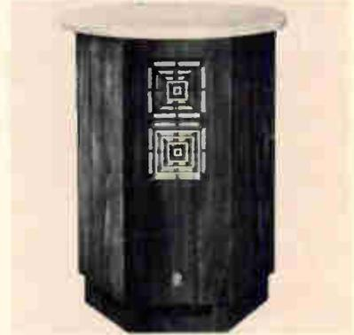
direct radiator mid-range, and direct radiator ultrasonic tweeter; frequency response 30-20,000 Hz (reference not stated); tweeter level control; 8 ohms nominal impedance; 75 watts (dynamic) maximum input power; dimensions 24 3/8" H x 18" diameter column; walnut finish with marble top; approximate weight 60 lbs; price \$109.95.
