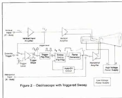
Figure 2 - Oscilloscope with Triggered Sweep
