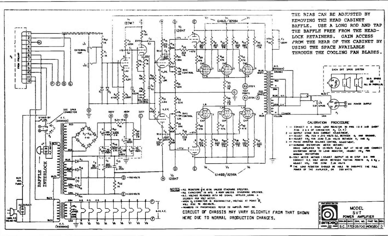
that's what you're seeking. I've tried the well-known 12AX7 conversion and found it changes the sound; I prefer the sound of 12DW7s. I find the General Electric 12BH7s to provide the fattest drive for the output stage. Try to find a matched pair—triode 1 should match triode 1 of the other tube in transconductance and cathode current. Triode 2s should also match.
