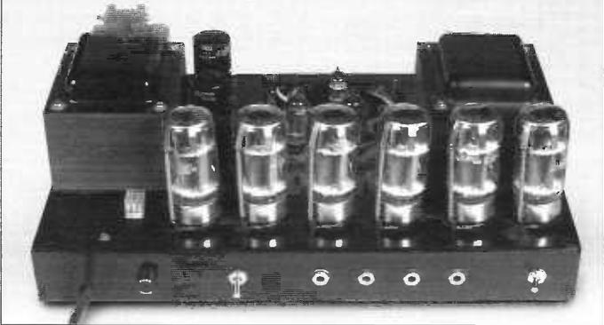
levels. While the 6146B/8298As held up to the mechanically abusive environment of taxi cabs, they were shown to be less tolerant of the abuse provided by the Rolling Stones—they would self-destruct when pushed into clipping for extended periods. Which, of course, the Stones did continuously. The SVT would soon be redesigned for six 6550 beam power tubes.
