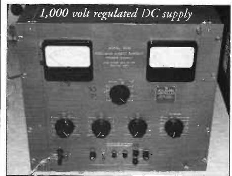
driver stage is obtained by using a standard radio-type power transformer running into a voltage doubler. The 6AX4GT damper tube rectifiers give a nice slow turn-on. The 6AX4GT is abundantly available in North America as a surplus TV tube.
