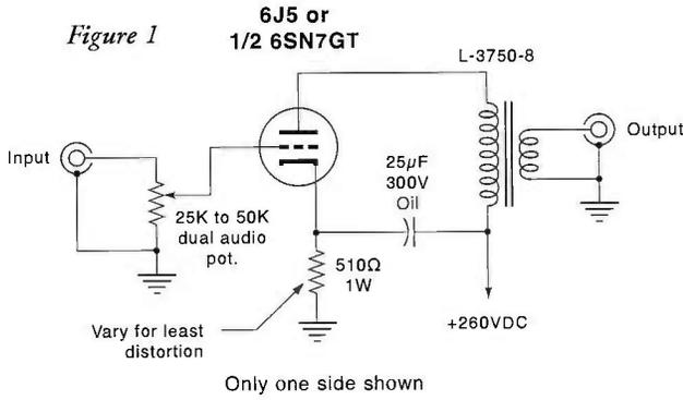
each tube will determine the secondary impedance, that is, a loaded secondary will reflect back to the plate load. This will need to be optimized with each tube type, but as long as it is higher that it needs to be, all should work well with a line output transformer such as the L3750-8. Frequency response will vary only slightly
