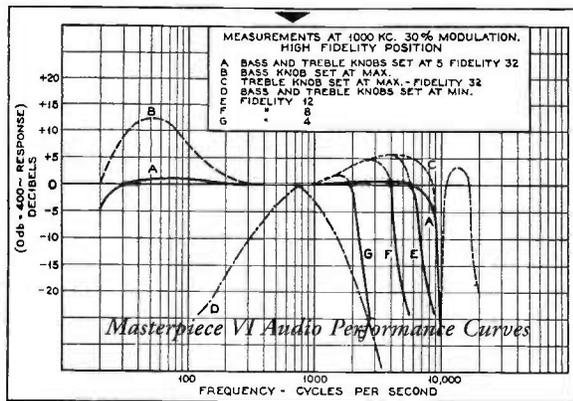
Fidelity Receiver (AKA Allwave 23 or Imperial), with its continuously variable IF selectivity of 2 to 32 kc (1 to 16 kc audio), was a superior performer.
