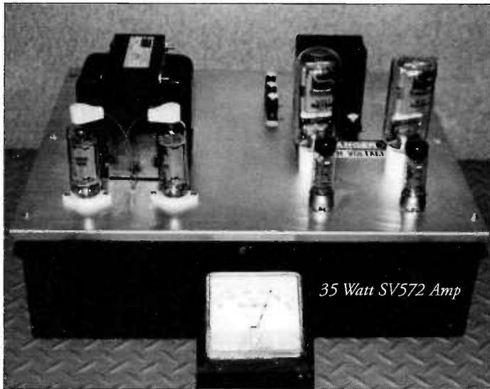
of failure, as the SV572-3s warm up far more quickly than the 6D22Ss. This diode is unusual in that it has a cathode cap rather than a plate cap. A connector for the cap with an insulating boot is recommended. The Svetlana PC509 has a ceramic body which completely covers the cap; nevertheless, if safety is an issue here, a cage over the tubes or an enclosed chassis is recommended.
