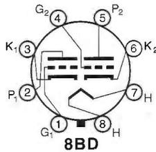
Why are we doing an article about this dual triode? It's not used in modern guitar amps, and it's not common in high-end equipment. This lack of use is not germane to its worth! The 6SN7 was a seminal audio type. First, it was the driver tube in the first American version of the Williamson amplifier. This was the first widely-used "hi-fi" amplifier design of the postwar era. Second, a good 6SN7GTB will give almost any other medium-mu triode a run for its money, in terms of linearity.
