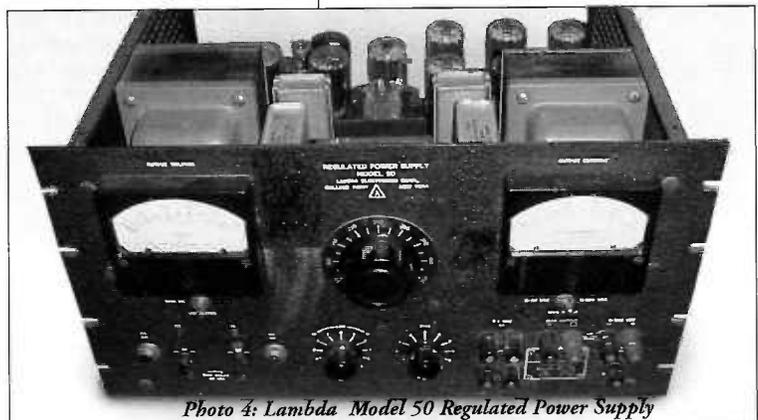
Photo 4: Lambda Model 50 Regulated Power Supply
