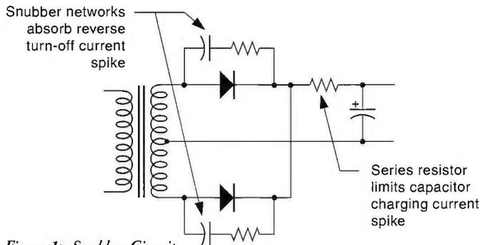
Figure 1: Snubber Circuit
