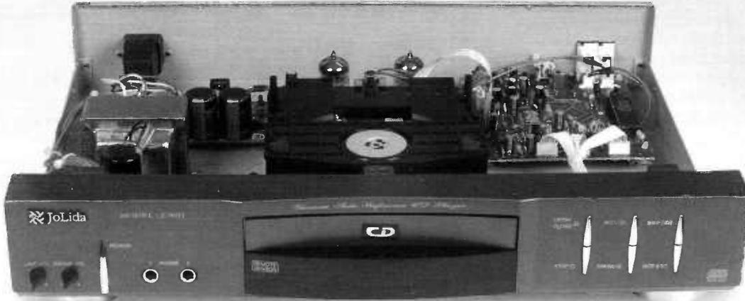
chip set. A couple of large high-quality coupling caps were also present in the analog stage. The chassis construction was nothing special, and no braces or attempts at vibration damping were evident.
