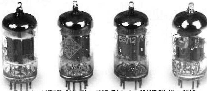
*Sylvania 12AX7WA Ring Plate 1987, Telefunken 12AX7 Rib Plate 1960s, Telefunken 12AX7 Smooth Plate 1960, JJ/Tesla ECC83 1990s*
