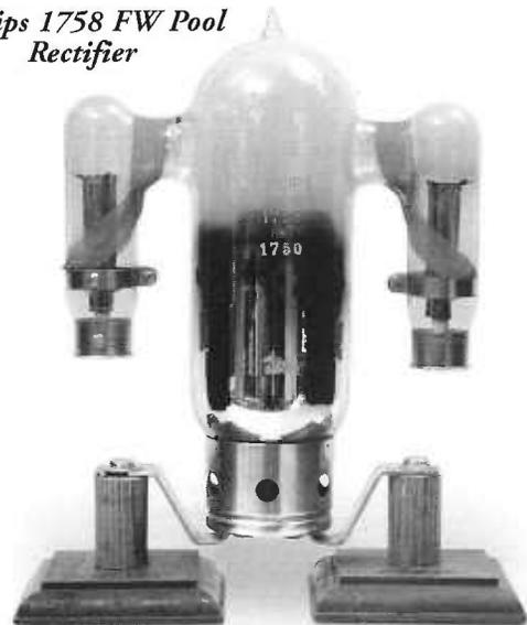
the small mercury pool in the bottom via an extra arcing electrode. Often made in low-voltage form, for lighting systems (12 or 24 volts), pool rectifiers were usually full-wave (in fact, variants were made with up to six, and even twelve, anode arms, for use with polyphase AC power systems), yet had a major disadvantage: occasional back-arcing could destroy the very equipment being powered. This has always
