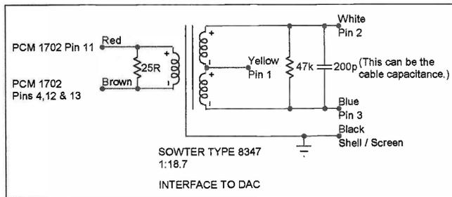
of 8.74k. This is in parallel with a 47k resistor placed across the secondary (per Sowter recommendation) giving a balanced source impedance of 7.4k or 1.84k for each phase. In balanced input mode, the minimum load presented is 2 X 51.1k, thus significantly greater than 10X the source impedance.
