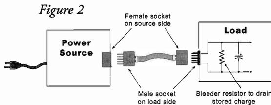
the scheme used in low-level audio connectors, such as XLR connectors. Don't mix hazardous voltages and audio signals in the same connector. This is good practice, not just for safety but for low hum and noise. UL and IEC require that any hazardous voltages on exposed terminals discharge to non-hazardous levels within two seconds of unplugging.
