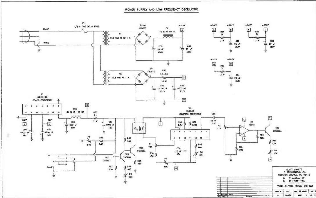
to implement. The chassis is connected to the buss at a single point. The input and output jack grounds are isolated from the chassis, connecting directly to the ground buss. The isolation can be accomplished by using plastic body jacks or using insulating shoulder washers. Using the concepts above, I had no hum problems with the unit. Hum and noise concerns are critical in an effects pedal since the signal strength entering and leaving is around 50 mV.
