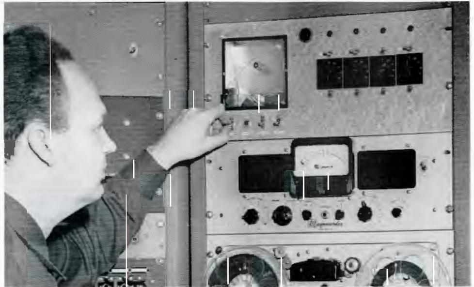
The author, Lyle Thompson, checks his cam-operated Automatic Starter Switch, used at Keating Studios to control the operation of a bank of Magnecorders which record NBC, ABC and MBS programs for Midnight Sun Broadcasting Company.
