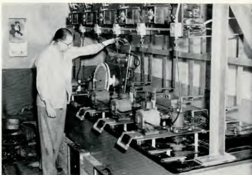
Plating technician Al Powers loads a silvered disc into the copper pre-plate bath where the first stage of the copper backing is applied in this automatically controlled, five unit tank. Discs are rotated while plating to assure uniform deposit.
