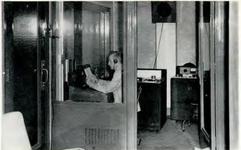
Recording and control room for Studio A, one of the special, acoustically treated reading rooms used for recording Talking Books. Mr. O'Donnell, of the recording staff, monitors the reading and keeps an eye on the Ampex console type unit as the story is taped.
