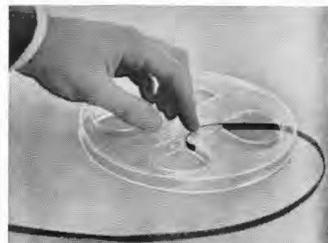
B. Drop tape into slot, leaving about 1 inch projecting beyond the hub with tape stuck on both sides of recording head. Then press the "start" button. Tape will grip and hold firmly . . . no need to turn reel by hand to anchor free end.
