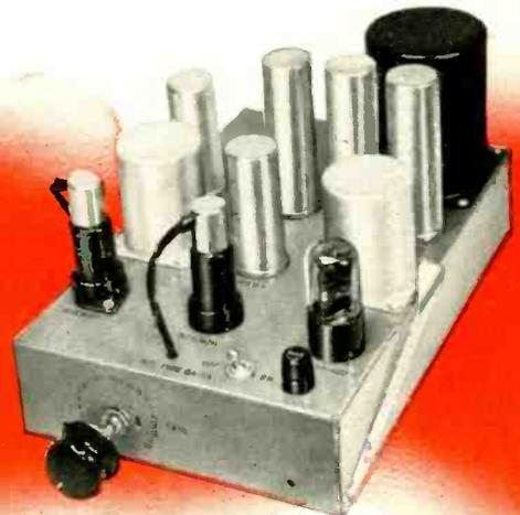
**Booster Amplifier (Type BA-2A)**—A two-stage unit having applications similar to those for the BA-1A; also valuable where a high-gain amplifier between announce microphone and limiting amplifier is required. *High gain:* 50 db. *Low noise level:* -68 db. *Low distortion:* 0.75% rms, 40 to 15,000 cycles. *Frequency response:*  $\pm 1.5$  db, 30 to 15,000 cycles. *Compact:* two units can be mounted on one 36-B or BR-2A shelf. Features plug-in capacitors and built-in power supply.
