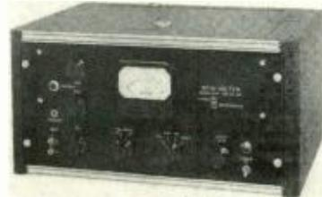
This instrument requires the use of a 1000 cycle phonograph record for testing phonograph turntables or equivalent signal sources for other recording and reproducing equipment. It consists essentially of an electronic frequency-meter, using one of the well-known circuits suitable for this
