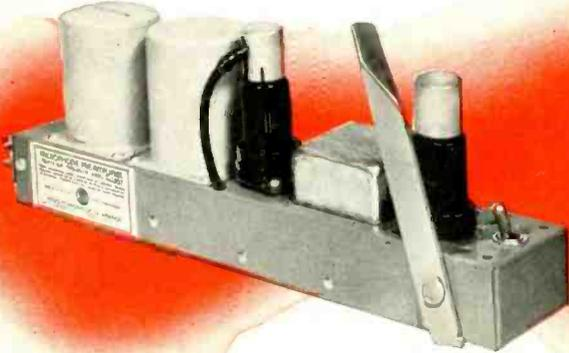
**Two-stage Preamplifier (Type BA-1A)**—ideal for use as a microphone preamplifier, turntable preamplifier, booster amplifier, or low-level isolation amplifier. *High gain:* 40 db. *High output:* +10 db. *Low noise level:* -80 db. *Low distortion:* 0.5% rms, 50 to 7500 cycles. *Isolation factor:* approx. 90 db; over 100 db with special Volume Control Kit. *Frequency response:*  $\pm 1$  db, 30 to 15,000 cycles. *Small size:* six units will fit on a 36-B or new BR-2A shelf!
