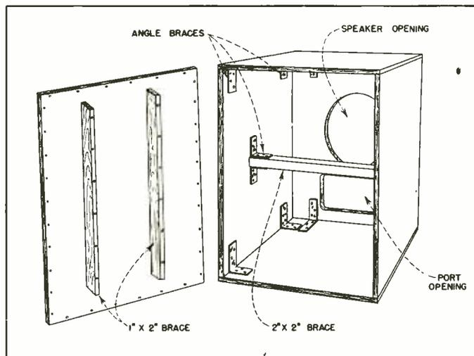
While the design of a suitable box may be done by means of a number of complicated formulas, the final result—as with anything in the audio field—is how it sounds when completed. Therefore, having decided upon a reasonable port size, it is much simpler to make the box and then experiment with the output until the result is satisfactory. This may be done by simple experimentation with the box, an amplifier, and an audio oscillator, in a method to be described later.
