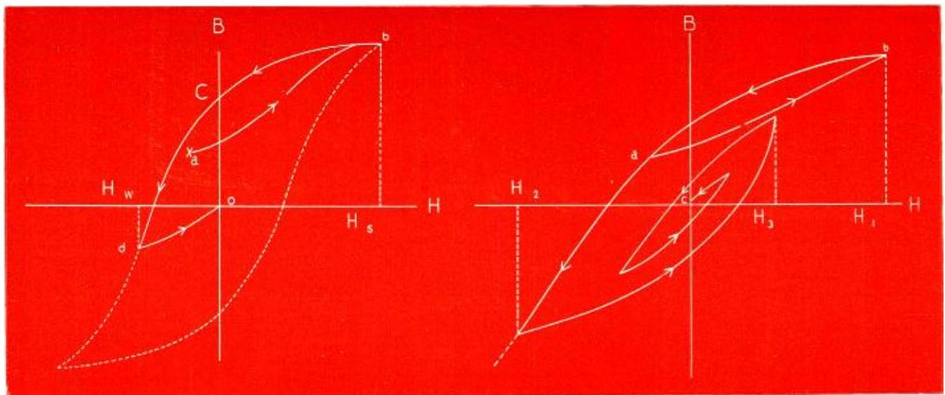
can result in noise levels below those of any usual amplifier may be attained by an a-c wipe. This form of erasure is stable in its final result and practical to apply. It is the form now generally employed.
