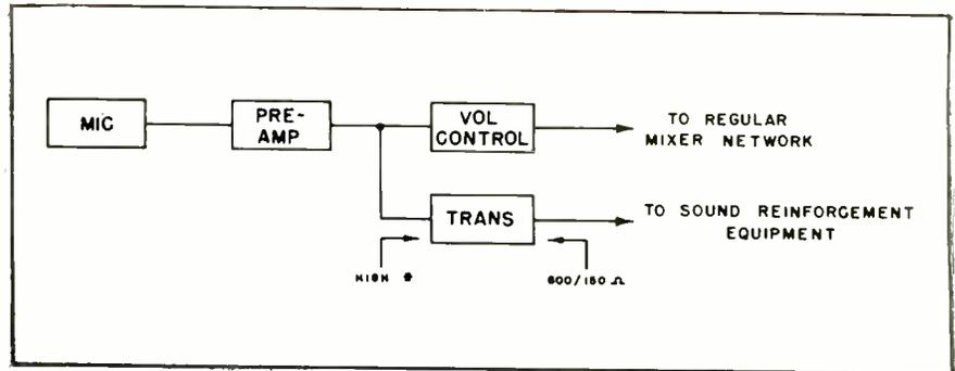
**Fig. 2.** Program feeds from the studio console to an external sound reinforcement mixer may be obtained by means of a bridging transformer, or bridging pad, connected across the output of the microphone preliminary amplifier as shown. If bridging pads are used several precautions must be observed as discussed in the text.
