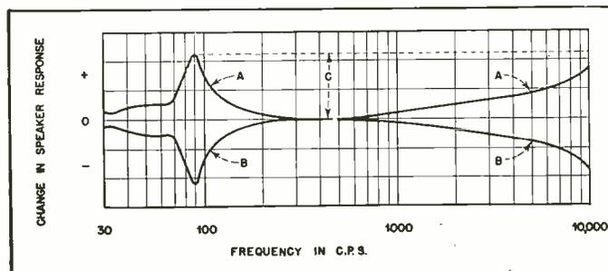
Fig. 1A. (top). Impedance characteristics of a typical cone speaker. Fig. 1B. Effect of amplifier on response of speaker with impedance shown in Fig. 1A. A. Connected to amplifier with output voltage regulation higher than used for original measurement. B. Connected to amplifier with output voltage regulation lower than used for original measurement. C. Maximum change cannot exceed the change in the amplifier output voltage regulation.
