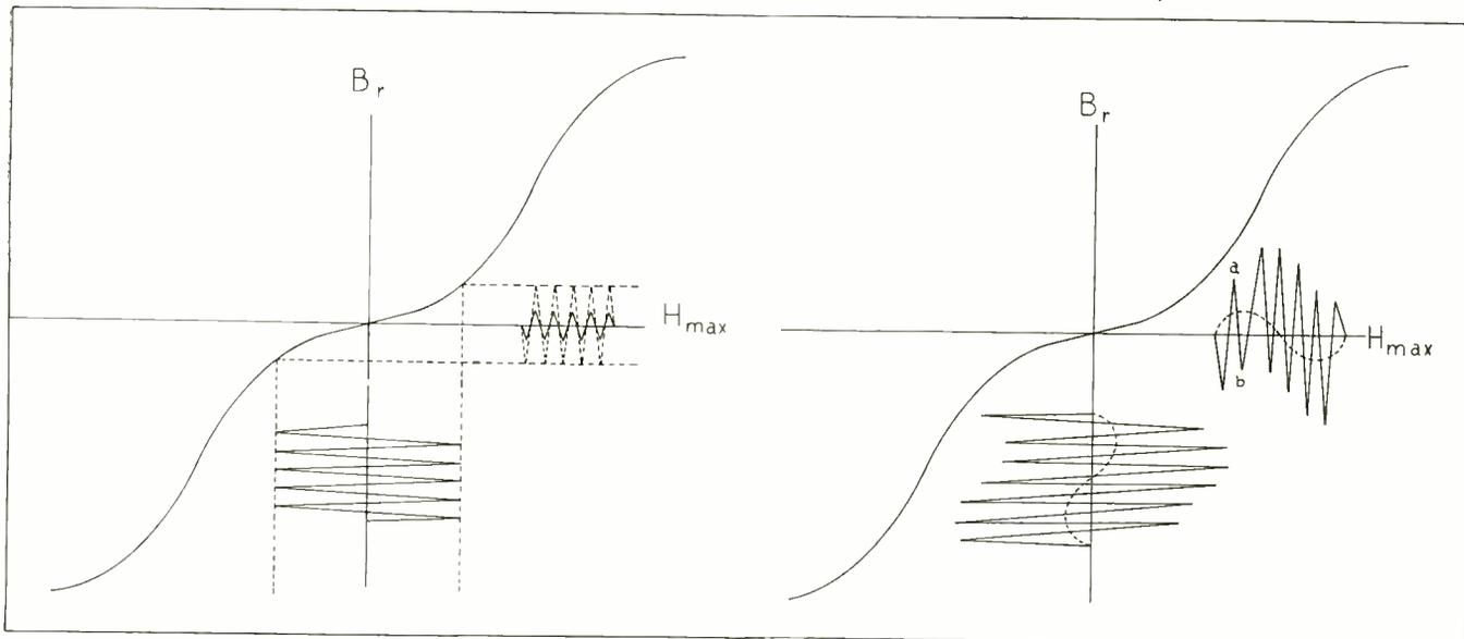
new frequency with an amplitude which is larger the greater the value of the recorded audio amplitude. This increase in amplitude is what would be expected if the demagnetization of the bias component of induction takes place according to the transfer characteristic curve for the bias frequency.
