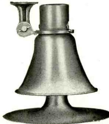
**NEW RADIAL RE-ENTRANT SPEAKER**, excellent for all types of industrial sound installations. Provides superlative and complete 360° speech intelligibility by efficiently over-riding factory high noise levels. Frequency response 300-6000 cps. Handling capacity 25 watts continuous, 35 w. peak. Has mounting bracket. Size 12" wide by 12 3/8" high.
