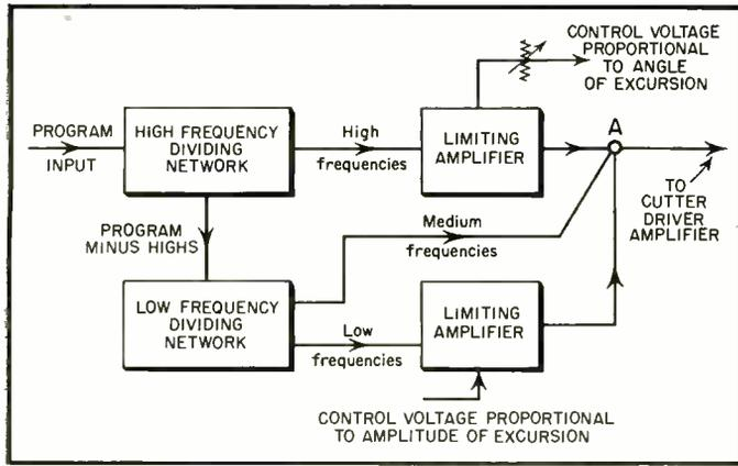
Fig. 2. Block diagram of essential Q-C circuit.
