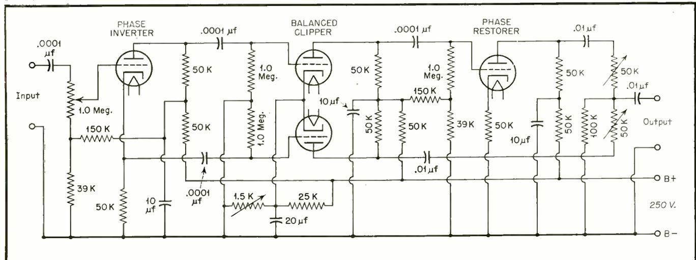
Fig. 5. This circuit may be employed to replace the transformer-terminated design shown in Fig. 3.
