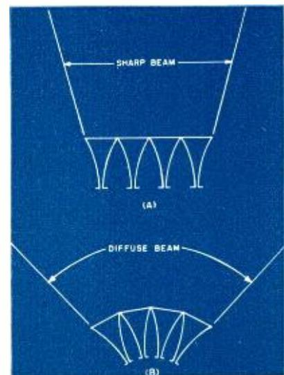
Fig. 14. Horn clusters: A.—For directivity. B.—For diffusion.
