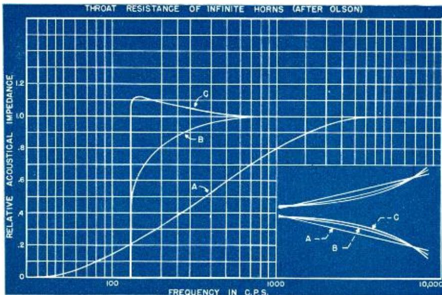
Fig. 11. Throat resistance of infinite horns (after Olson).
