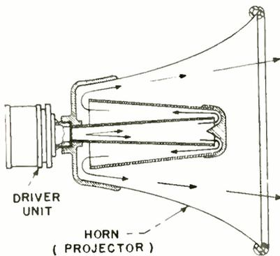
Fig. 13. Re-entrant horn.
