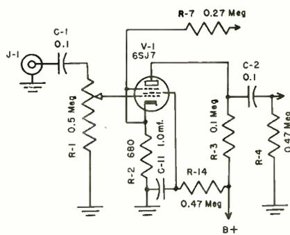
Fig. 5. Schematic of changes to circuit of  $V_1$  when used as a pentode for increase of approximately 20 db in gain. Only required changes are in cathode resistor  $R_2$  from 5,600 ohms to 680 ohms, and addition of  $R_{14}$  and  $C_{11}$ . No change is necessary in feedback resistor,  $R_7$ .
