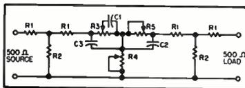
Fig. 3. Basic circuit of combined NAB and radius-equalizing networks. (Values explained in text.)
