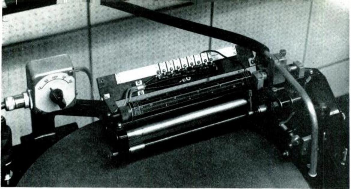
Fig. 2. Automatic radius-equalizer fabricated for Fairchild 199 recorder. Control switch is located at left of equalizer.
