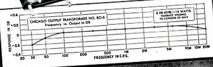
**No. BO-6.** For use in high fidelity amplifiers. Couples push-pull 6L6's (7500 ohms, C-T) to 6/8 or 16/20-ohm voice coil. Center-tapped tertiary winding provides 15% inverse feed-back to reduce harmonic distortion to a minimum. In drawn steel case, 4 $\frac{1}{16}$ " x 3 $\frac{3}{8}$ " x 3 $\frac{1}{16}$ ", with mounting studs and convenient pin-type terminals . . . List Price, \$23.00
