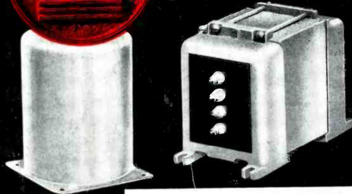
U.T.C. Commercial Grade components employ rugged, drawn steel cases for units from 1" diameter to 300 VA rating . . . vertical mounting, permanent mold, aluminum castings for power components up to 15 KVA. Units are conservatively designed . . . vacuum impregnated, . . . sealed with special sealing compound to insure dependability under continuous commercial service.
