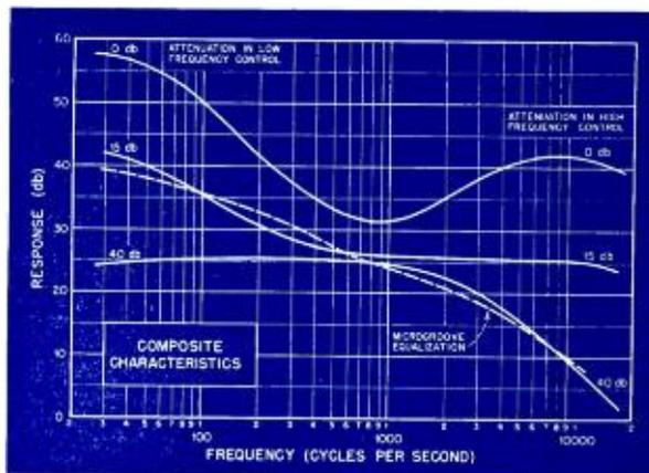
Only three characteristics are shown in *Fig. 4*. Two of these represent extremes, with either no attenuation, or large attenuation, in both auxiliary channels. Between these extremes is a large number of possible characteristics, of which only one is illustrated.
