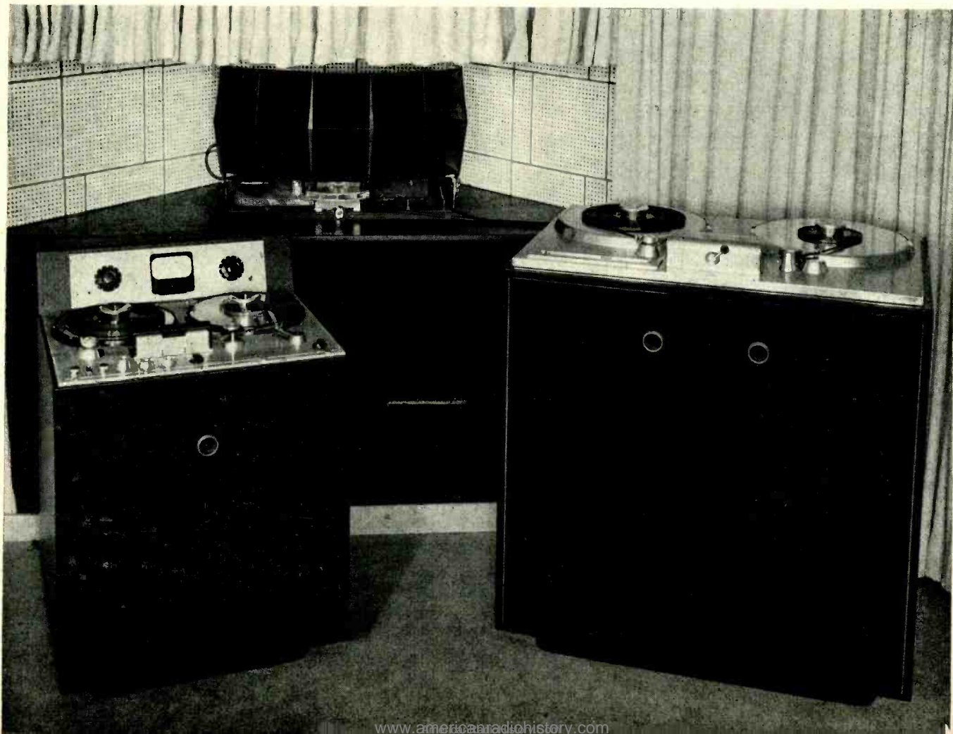
Fig. 3. Model 300 recorder (left) beside the Model 200, illustrating the reduction in size in the new unit. Also shown is the extended-range speaker system used for critical listening tests. The unique Smith-Selsted tweeter (center) provides flat response up to 20,000 cps.
