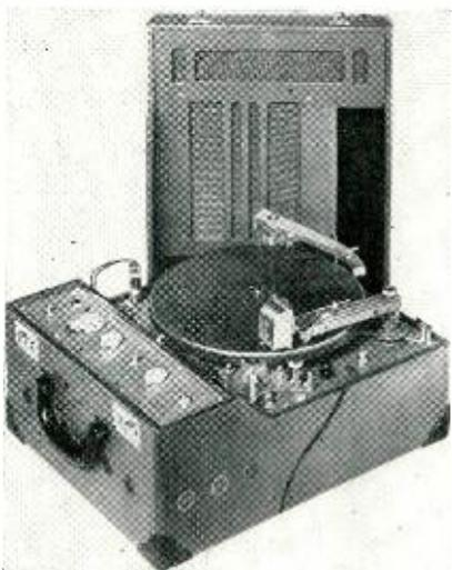
which are modifications of the famous Presto K-8 and Y-2 types. The new units will do standard recording as well as Microgroove, and modifications include an advance ball on the cutting heads and dual purpose pickups. The quality of recording is excellent. The K-8 will record continuously for one-half hour on one side of a 13 1/4" disc. Microgroove units are offered at no price increase over former types.
