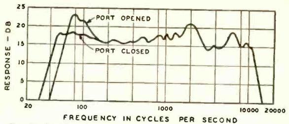
Fig. 10 (right). The overall response-vs-frequency characteristics of the duo-cone speaker in the cabinet of Fig. 8 with the port open and closed.
