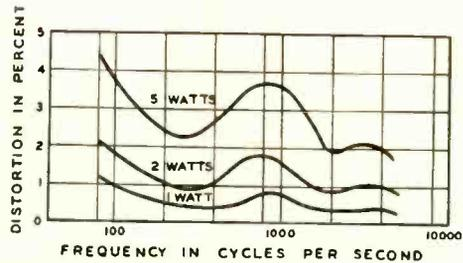
Fig. 13 (right). The total nonlinear distortion-vs-frequency characteristics of the duo-cone speaker for inputs of 1, 2, and 5 watts.
