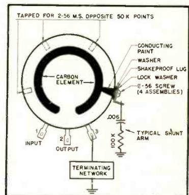
Fig. 2. Physical modifications to standard type of volume control to convert to loudness-control operation.
