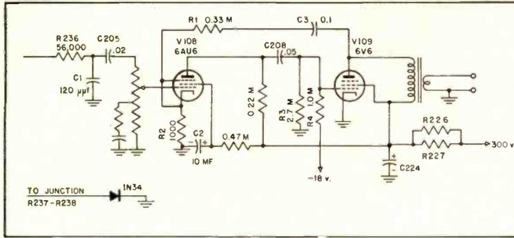
Fig. 2. Recommended changes, using feedback from plate of output stage.
