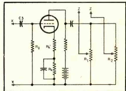
Fig. 6. Alternate use of tube instead of transformer to provide necessary phase reversal.
