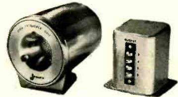
This compact "super tweeter" originated in the h-f channel of the famous Jensen G-610 Triaxial. Makes an excellent "top end" for custom-built multi-channel systems. No installation problems. Simple to mount. Provides smooth, clean highs from 4,000 to approx. 18,000 cycles with extremely low distortion. **Model RP-302 \$32.93 Net**
