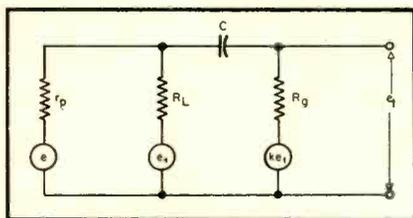
Fig. 2. Equivalent circuit of amplifier shown in Fig. 1.
