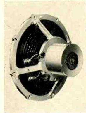
sion of the cone. The Super 5 is supplied mounted on an 8-by-8 in. plywood board with 3½-in.-diameter aperture, which is the effective cone diameter. May be used with two-speaker systems employing 1000-cycle crossover merely by connecting in parallel with the present treble unit and by inserting a 0.5-µf. capacitor in series with the voice coil of the Super 5. British Industries Corporation, 164 Duane St., New York 13, N. Y.
