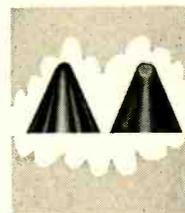
**Record Wear** is hard to detect except by comparison. A wearing stylus tip (right) shows gradual distortion. Diamond stylus (left) runs hundreds of hours without visible wear. Easy to buy and install, the diamond pays off in listening pleasure and record protection.
