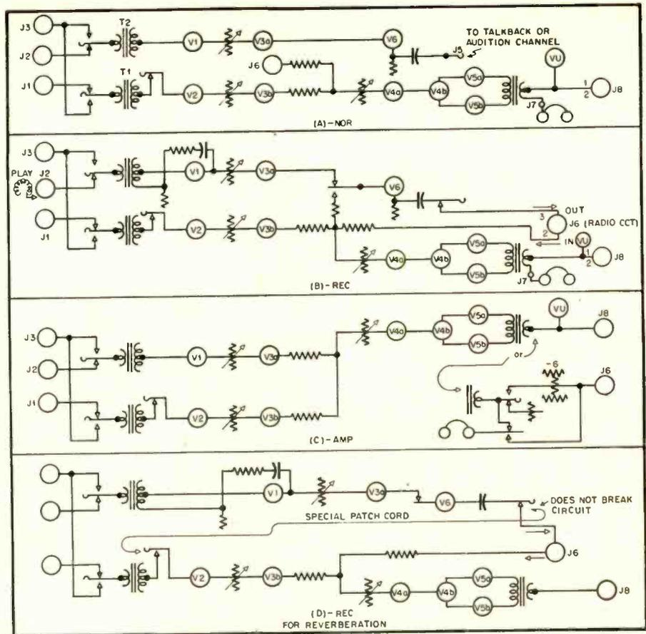
Fig. 4. Block schematic of the amplifier for the three positions of the selector switch, SW<sub>a</sub>, b, c, d, and when connected for reverberation. When connected to a home music system,  $J_6$  is shorted so the unit is out of the circuit when the selector switch is at NOR.
