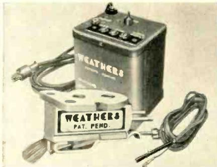
tube. Oscillator output is 0.5 volt at high impedance—can be fed into crystal or tuner input of any high-quality amplifier. Power required is 6.3 volts a.c. at 0.3 amp and 250 volts d.c. at 2 ma, which may be obtained from amplifier or from Weathers power supply which is available as an accessory. Weathers Industries, West Collingswood, N. J.
