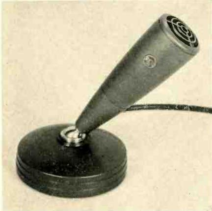
obtrusive gray for TV. The BK-1A is a pressure-type microphone in which voltage response is made nearly independent of frequency by coupling acoustic circuits to the diaphragm. Frequency response is 60 to 10,000 cps. and effective output level is -53 dbm. In most respects the BK-1A duplicates RCA's popular Model 88-A, which it replaces. However it is much more suitable for TV because of improved appearance. RCA Victor Division of Radio Corporation of America, Camden, N. J.
