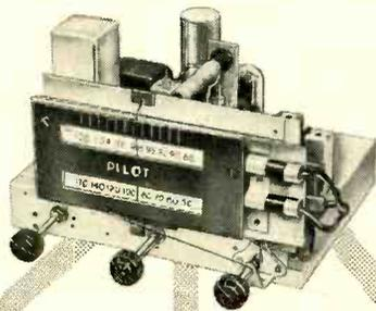
rule dials for AM and FM, tuned RF stage on FM for maximum sensitivity and selectivity, temperature compensated oscillator, ratio detector with 225 Kc wide linear response, IF response 200 Kc wide at 6db points, 300 ohm input. Low output impedance. Phono and TV inputs controlled by switch. 9 miniature tubes plus rectifier. Controls: Band Switch, On/Off/Volume, Tuning.
