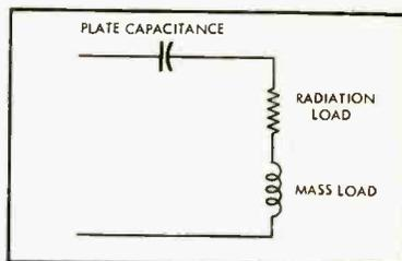
Fig. 2. The basic impedance elements in an electrostatic loudspeaker unit. This is not complete, but shows the principal elements.
