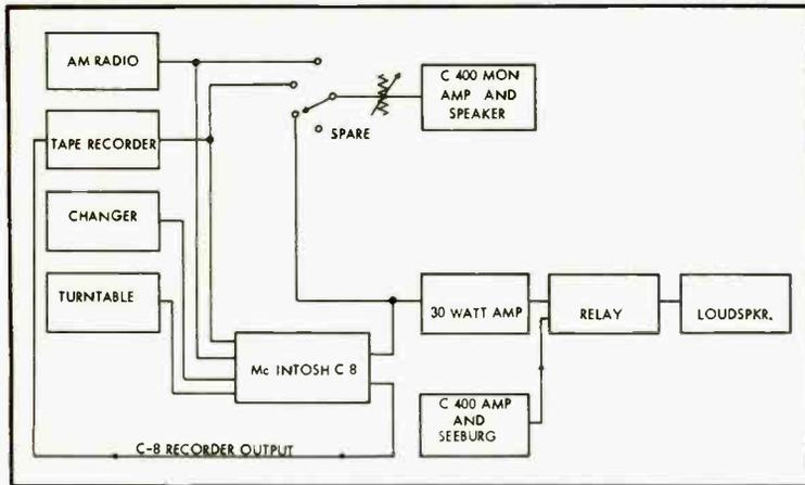
Fig. 1. Block diagram of the control room equipment used in the college music room.
