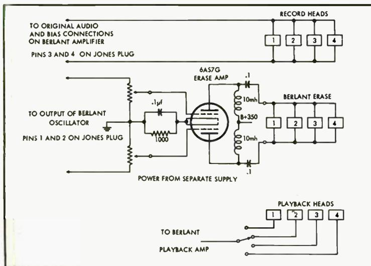
Fig. 4. Using one erase oscillator and an erase amplifier enables the station to employ only one amplifier to record on four machines simultaneously.
