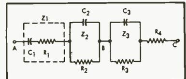
Fig. 13. Circuit of Fig. 12 redrawn for purpose of analysis.
