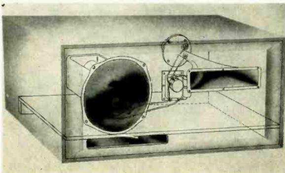
Fig. 4. Internal construction of the small system.
