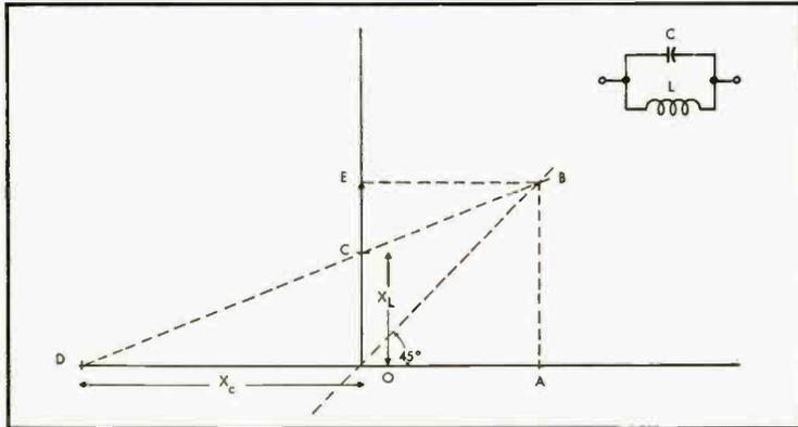
Fig. 10. Construction for capacitance and inductance in parallel.
