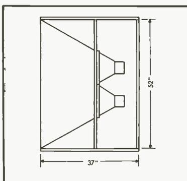
Fig. 3. Section through A-A of Fig. 2 to show flare at top and bottom of main horn.
