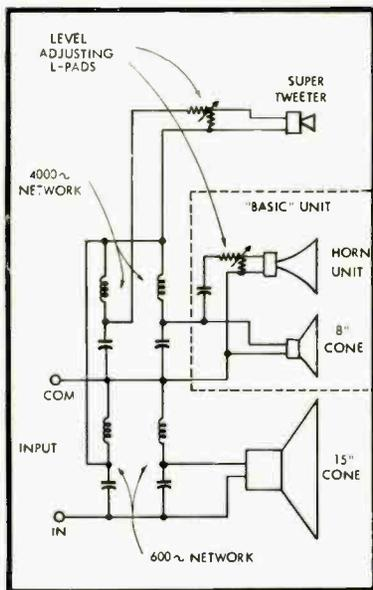
Fig. 3. Simplified schematic of the complete system. Section enclosed in dotted lines is the system in the small cabinet. Individual level-adjusting controls make it possible to balance the system quite accurately, although the balance between the 15-in. woofer and the lower-midrange 8-in. cone depends upon the built-in sensitivity of the two mechanisms.
