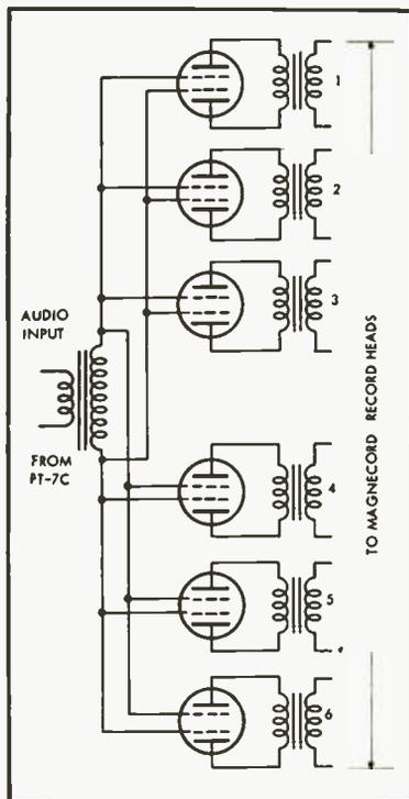
Fig. 1. Six separate output stages fed by the same input transformer eliminate the problem of interaction between bias circuits.
