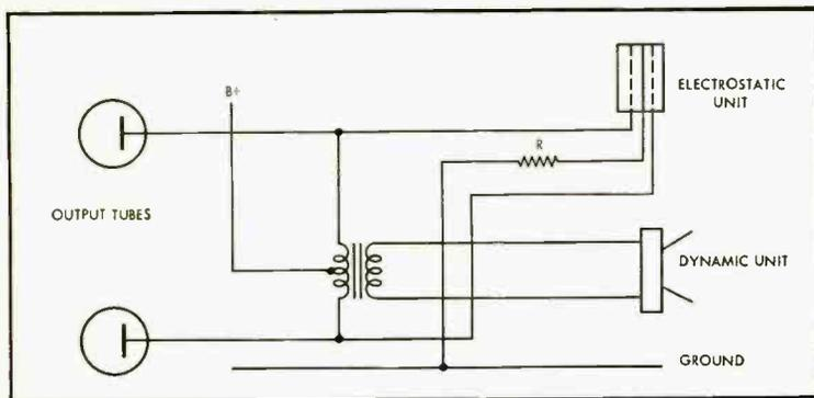
Fig. 3. Basic method of connecting a dynamic and an electrostatic unit to the same amplifier output as a two-unit system.
