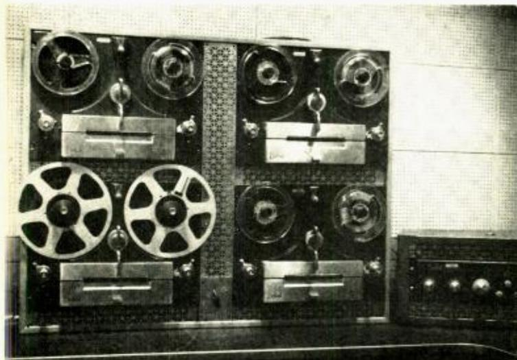
Fig. 3. Four Berlant tape-transport mechanisms and one amplifier comprise new setup giving same advantages over older equipment.
