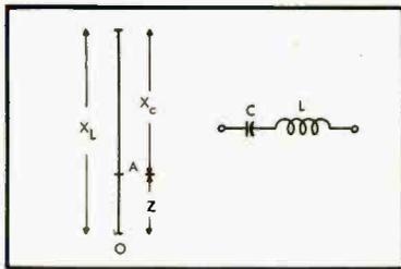
Fig. 9. Inductance and capacitance in series involve only vertical straight lines.
