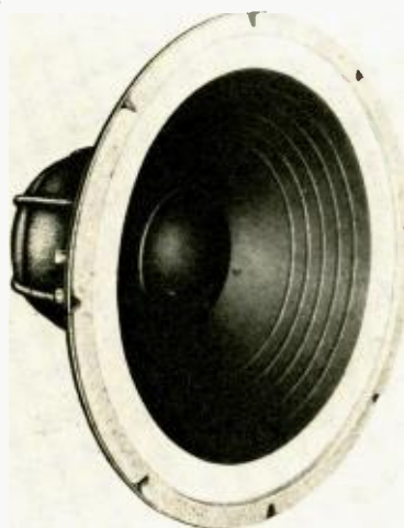
Fig. 1. 15-in. woofer having high compliance cone, with plastic foam surround. Resonant frequency is 24 cps.
