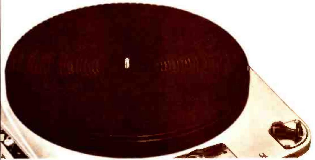
The 301 turntable weighs a full 6½ lbs. and it is made of precision-machined cast aluminum. Being heavy and dynamically balanced as well, it imparts flywheel action, which tends to override a variation in speed.
