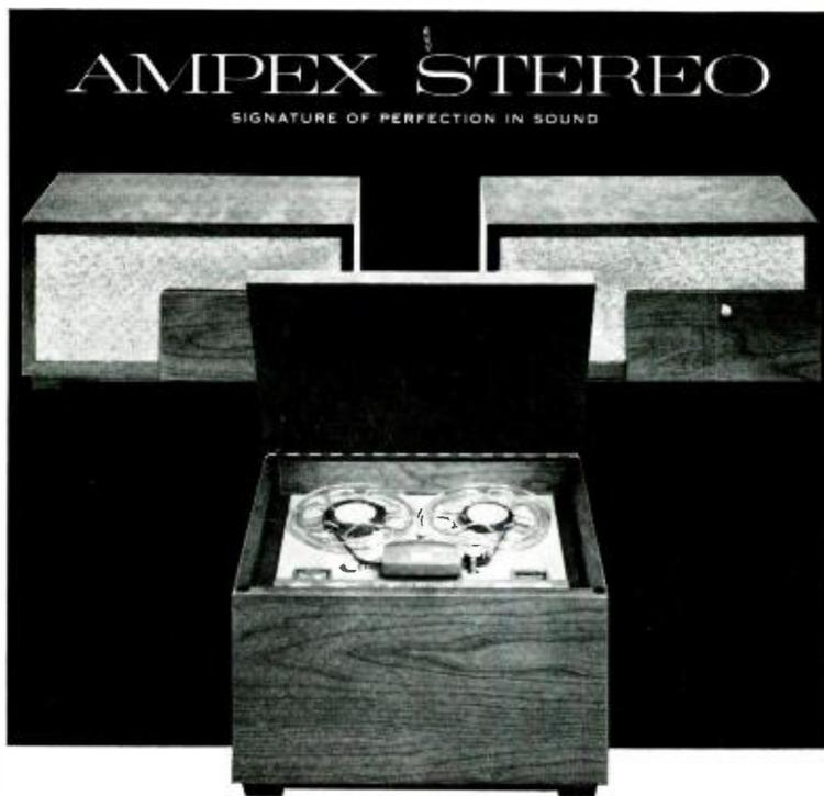
**Recorder-Stereophonic Reproducer**—Two-speed, precision-built tape transport, capable of playing over 4 hours from a single 7" reel of tape; sustained frequency response 30-16,000 cps (7½ ips), with dynamic range over 55 db; Flutter and wow under 0.25% rms at 7½ ips; Precision timing accuracy affords perfection of pitch held to tolerances of less than 1/3 of a half tone at highest frequencies.
