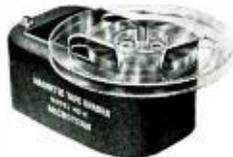
Erases recorded signals and noise from magnetic tape without rewinding. Spindle mounting of reel permits rapid coverage without missed spots. Noise level reduced below level of standard erase heads. Restores tape to like new condition or better. Reel size range 5", 7", 10 $\frac{1}{2}$ ". May also be used for demagnetizing record-playback-erase heads.
