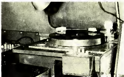
Fig. 4. Disc recorder for location cutting of test discs. Note remote control buttons for the tape recorders in mounting just to left of console.
