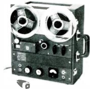
head which permits playback flat within  $\pm 2.0$  from 10 to 15,000 cps. The drive mechanism is powered by a hysteresis synchronous motor which holds wow and flutter well within professional standards. A two-speed unit, the 90-S may be operated at 7.5 or 3.75 ips in either horizontal or vertical position. An illuminated VU meter and an index counter facilitate recording and location of desired program material on a spool of tape. Timing ac-
