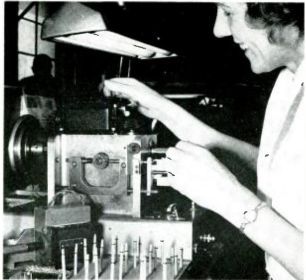
Fig. 6. Coil winding machine for pickup coils.
