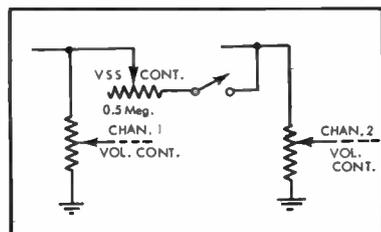
Fig. 1. Simple variable-stereo-suppression control.
