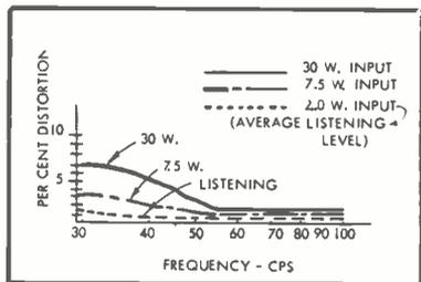
Fig. 5. Distortion of woofer at various power levels.
