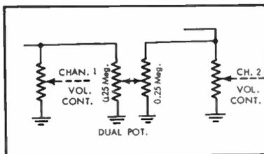
Fig. 2. Self-isolating variable-stereo-suppression control. The central ground permits no "bleeding" of channels when the control is at minimum.
