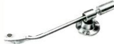
friction-free vertical and horizontal movement. Open-front design permits visual location of stylus in record groove. While mechanically a single unit, the arm is divided into two sections isolated acoustically from each other. Resonance varies from 12 to 15 cps, depending upon the cartridge employed. Rek-O-Kut Company, Inc., 38-19 108th St., Corona 68, N.Y. H-47
