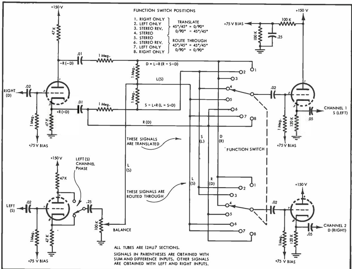
Fig. 1. Schematic of multipurpose device for complete control of all types of stereo signals.
