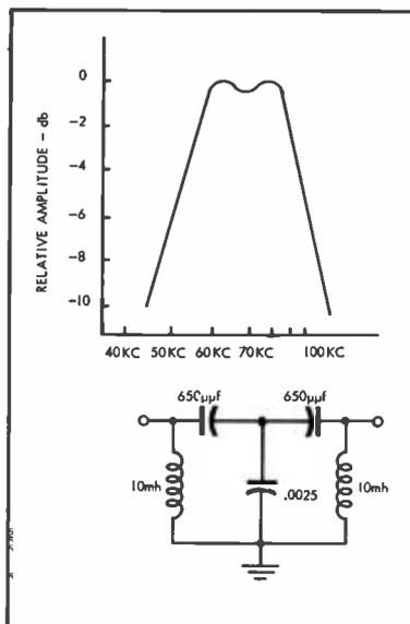
Fig. 8. This band-pass circuit can be used following or to replace the high-pass filter if it is found necessary for the 67-kc subchannel. Its purpose, as shown in the response curve, is to limit the response of the amplifier to noise lying above 80 kc.
