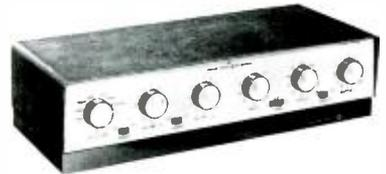
are included for monophonic use. Frequency response is 20 to 20,000 cps  $\pm 1.0$  db. Controls include bass and treble, scratch filter, rumble filter, loudness switch, and mono-stereo and channel-reverse switch. All filaments are operated on d.c. to ensure minimum hum. Ten inputs are provided for virtually every type of signal source, including microphone. Allied Radio Corporation, 100 N. Western Ave., Chicago 30, Ill. H-30
