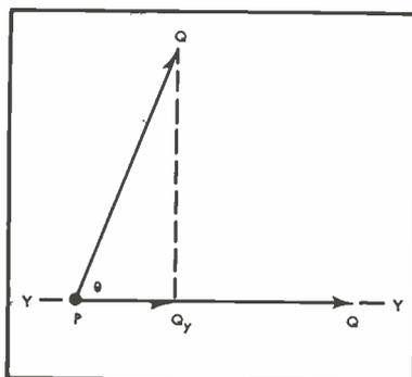
Fig. 1. Vector diagram of effect of noise on a monophonic pickup.
