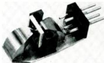
Fig. 7. Assembly of pickup to show magnet structure.
