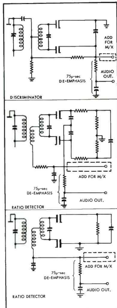
Fig. 2. FM detectors of three typical commercial receivers indicating proper point to connect the multiplex output. The connection is always made just before the de-emphasis network. In each case there still remains a small capacitor shunting the MX output to ground. It serves to bypass the 10.7-mc carrier, and does not interfere with the MX signal.
