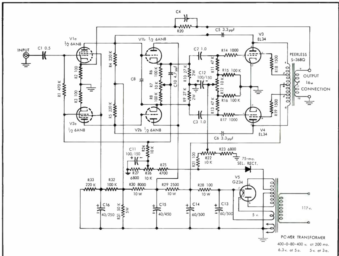
Fig. 5. The complete amplifier using a pair of EL34's in the output stage reaches a new low in distortion and unbalance.
