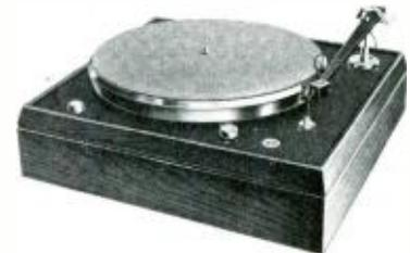
Stereotable is a single-speed machine—33 1/3 rpm—and incorporates a built-in precision leveling adjustment. Vertical period of spring suspension is below 5 cps, and compound vertical rumble attenuation is 12 db/octave below resonance. Noise is 65 db below reference level, and speed accuracy is  $\pm 2.0$  per cent total variation. Pickering & Company, Inc., Plainview, N.Y. H-46
