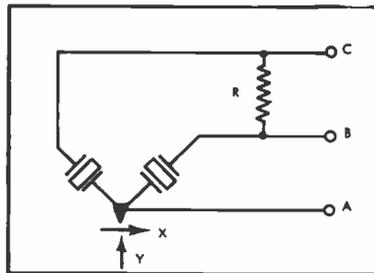
Fig. 3. Simple method of mixing lows with a ceramic pickup to decrease the effect of rumble.
