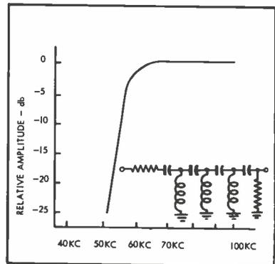
Fig. 7. Frequency response before limiter when set for 67-kc subchannel.
