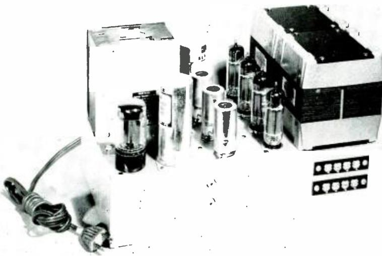
Fig. 1. Combining two 15-watt amplifiers onto one chassis results in a stereo "package" which compares favorably with most any amplifier available.
