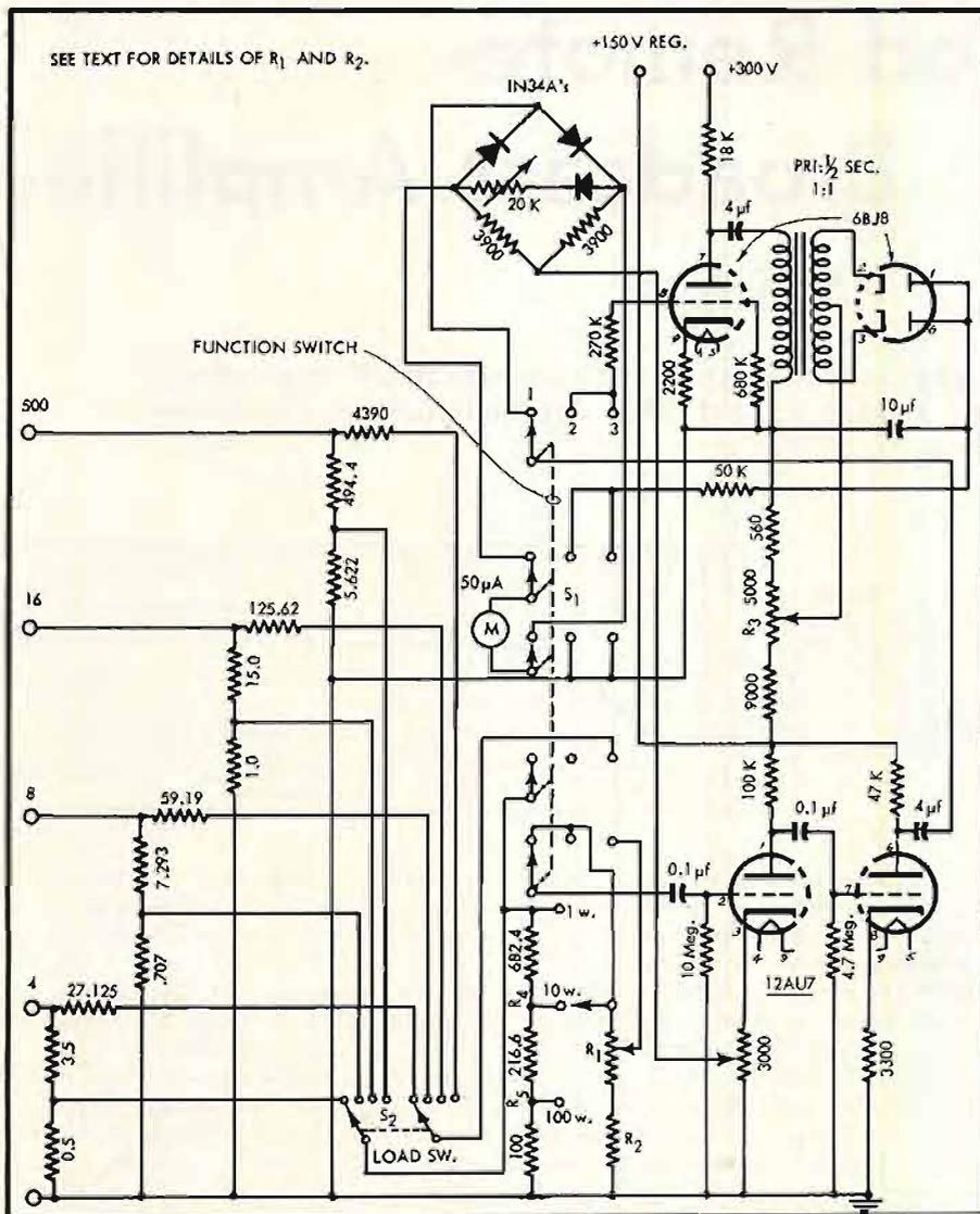
Fig. 3. Complete schematic of direct-reading damping-factor meter.
