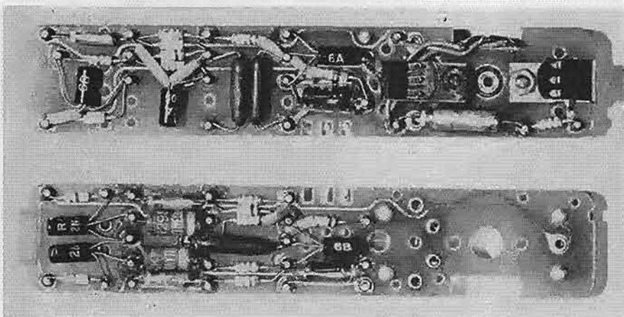
Fig. 7. Details of the two printed-circuit sections which are mounted back to back.
