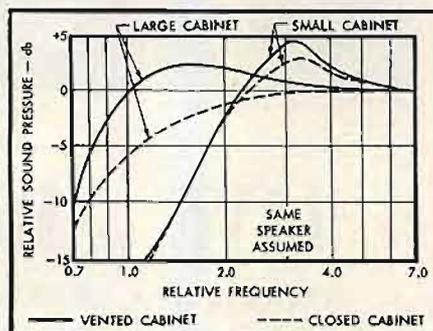
Curves here show how the smaller air stiffness of the large box allows lower system resonance. The inevitable 6-db-per-octave dropoff below resonance can be then set below the listening region instead of in it. Thus amplifier power or distortion will not increase to maintain flat output over the entire listening region.
