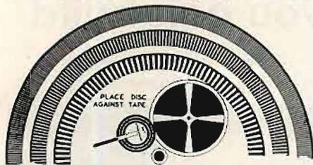
6041, Montgomery 6, Ala. The disc is mounted on watch-type bearings to eliminate drag. Total weight of the assembly is only five ounces. The disc indicates three speeds— $3\frac{3}{4}$ ,  $7\frac{1}{2}$ , and 15 ips. It must be used in conjunction with a 60-cps a.c. light source. **A-1**
