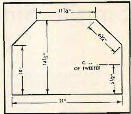
Fig. 2. Physical measurements of the Rebel IV enclosure.
