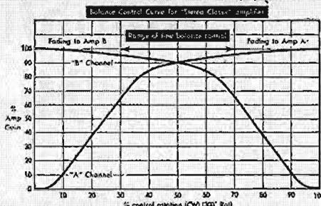
**Versatile, convenient switches and controls.** In this completely new and striking General Electric design you'll find every useful variation in stereo and monaural amplification, controlled swiftly and accurately. Balance control allows you to adjust for maximum stereo effect *without* overloading one channel when the other is cut down. New contour control boosts the bass smoothly, gradually, *without* increasing sound intensity. Each control handles *both* 20-watt channels.
