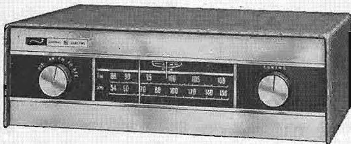
**Top performance in a trim, modern cabinet.** Receives even weak signals with unusually low distortion, hum and noise level. No audible drift. Visual meter provides center channel tuning of FM and maximum AM signal. RF amplifier stage in both FM and AM for increased sensitivity. FM multiplex jack for stereo adaptor. Built-in AM antenna; folded FM dipole included. **\$129.95\***.
