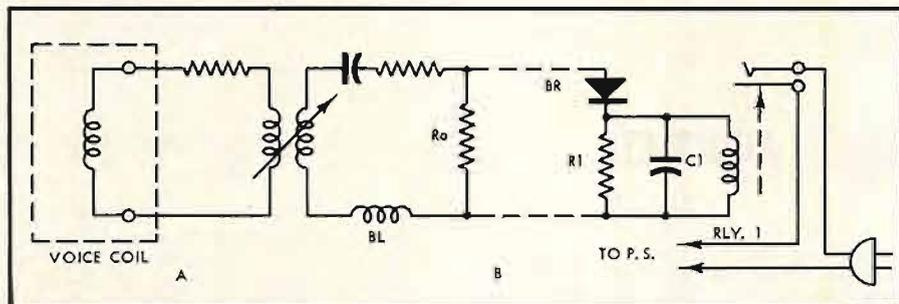
Fig. 4. Feedback-type network to actuate cut-off relay.
