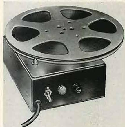
and removed to a distance of at least six feet. The degausser incorporates two transformers drawing 6 amps at 110 vac, an on-off switch, and a line fuse. Dimensions are  $6\frac{1}{4}$ "  $\times$   $7\frac{3}{4}$ "  $\times$   $3\frac{1}{2}$ ". Carrying catalog No. ML-120, this unit is available from Lafayette Radio, Jamaica 33, N.Y. **A-6**
