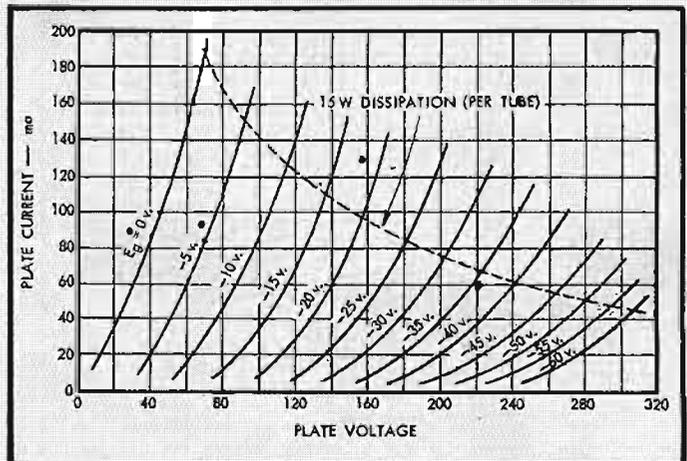
Fig. 3. Plate family for the 5998 tube.
