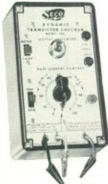
and NPN models. If desired, similar transistor types can be effectively matched. The unit is powered by a self-contained 1.5-volt battery and utilizes a Type NE-51 glow lamp as the visual signal to indicate test results. Compact and portable, the tester measures just 3 1/4" w x 6 1/4" l x 2 1/4" d, and weighs 1 1/2 lbs. For detailed specifications write Seco Manufacturing Company, 5015 Penn Ave., S., Minneapolis, Minn. **B-1**
