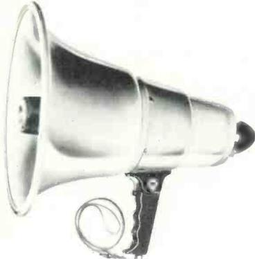
portable p.a. system. Constructed of lightweight aluminum, the Megavox is equipped with a waterproof magnetic microphone and is usable under any weather conditions. Powered by three standard NEDA Type 706 4.5-volt batteries, it incorporates a class B transistorized 5-watt push-pull amplifier, and is equipped with a pistol-grip trigger switch and variable volume control. **Fanon Electronic Industries Inc., 98 Berriman St., Brooklyn, N. Y. B-8**
