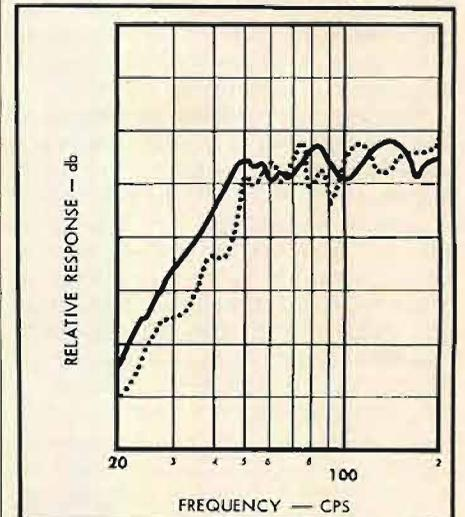
Fig. 5. Low-end response of Bi-Phonic Coupler (solid curve) vs. a conventional low-efficiency, long-throw, low-resonance piston in a sealed acoustically-stiffened box.
