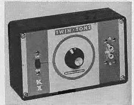
ready for immediate use. By sliding a switch located on the front panel, a constant 1000-cps tone is produced. The volume controls on the amplifier are then adjusted until the speakers have identical output. A volume control permits adjusting the signal to any desired level. The Twin Tone is powered by an internal mercury battery. Kinematix, Inc., 1616 N. Damen Ave., Chicago 47, Ill. C-11
