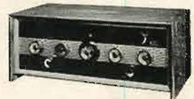
**Specifications:** Inputs: 3 high level; 2 low level • Outputs: 2—one main amp, one recorder • Gain: 60 db at 1 kc • Response: 20-22,000 cps • Noise level: 95 db below 1.5 v output • Controls: 7: switches for choice of inputs; separate volume, power, tape, bass and treble controls; 5 level controls • Power supply: self contained—117 v, 60 cycles • Dimensions: 4 $\frac{1}{2}$ " H x 13 $\frac{3}{4}$ " W x 5 $\frac{3}{8}$ " D • Weight: 11 lbs. Price: **\$147.00**
