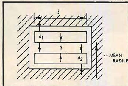
Fig. 14. Dimensions required for calculation of leakage inductance.
