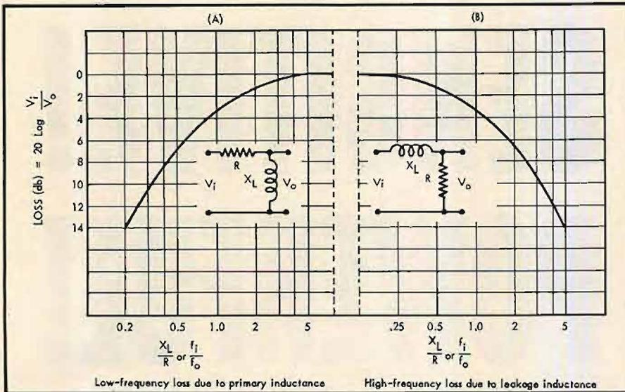
Fig. 7. Basic output transformer characteristics.  $f_o$  is the frequency at which the reactance  $X_L$  is equal to the resistance  $R$ , and  $f_i$  is the frequency at which the loss is to be determined.
