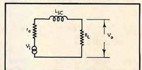
Fig. 12. Equivalent circuit at frequencies above 4000 cps.
