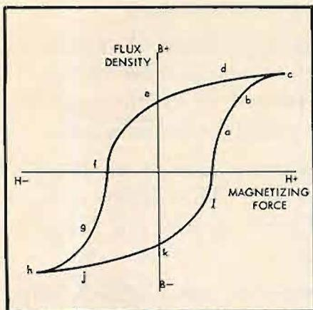
Fig. 16. Typical B/H relation for iron laminations.
