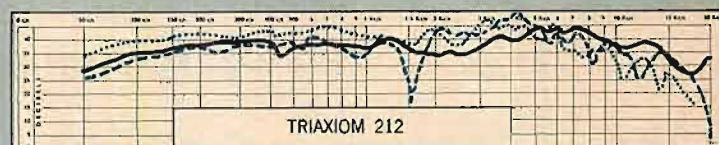
CONSTANT TEST CONDITIONS: Microphone 18" on axis. Anechoic conditions. Infinite baffle. Input, 1/2 watts at 400 cycles
