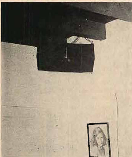
Fig. 5. Midrange horn disperses sound throughout the large room, augmented by a woofer at floor level.
