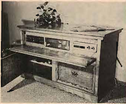
Fig. 3. Top edges of the console are covered with wood tape.
