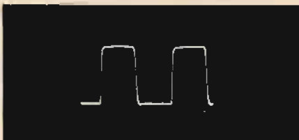
Fig. 8. Square-wave response at 10,000 cps.
