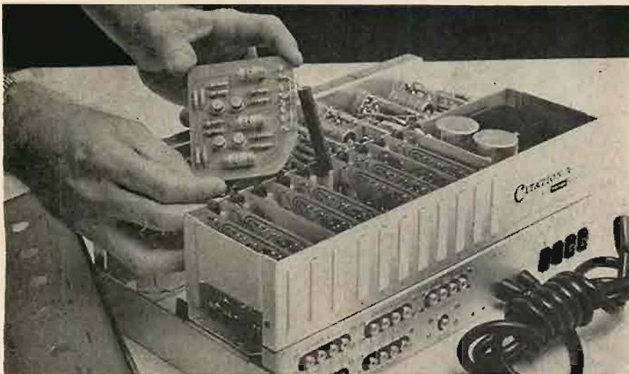
Fig. 2. View of the Citation A showing the housing for the eleven three-transistor modules, one of which is shown removed from the nylon "tracks" into which it fits.
