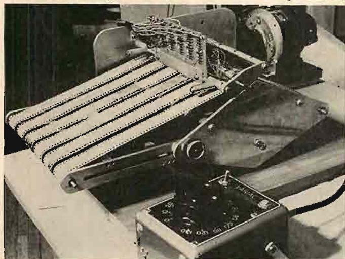
Fig. 7. The complete six-channel Hamograph. The variable-speed motor at the rear is controlled by the Variac in the foreground to change speed on all six tracks at once. Note resistors which attenuate bias are mounted on the feeler carriage. Wire placement is not critical since only d.c. voltages are involved.
