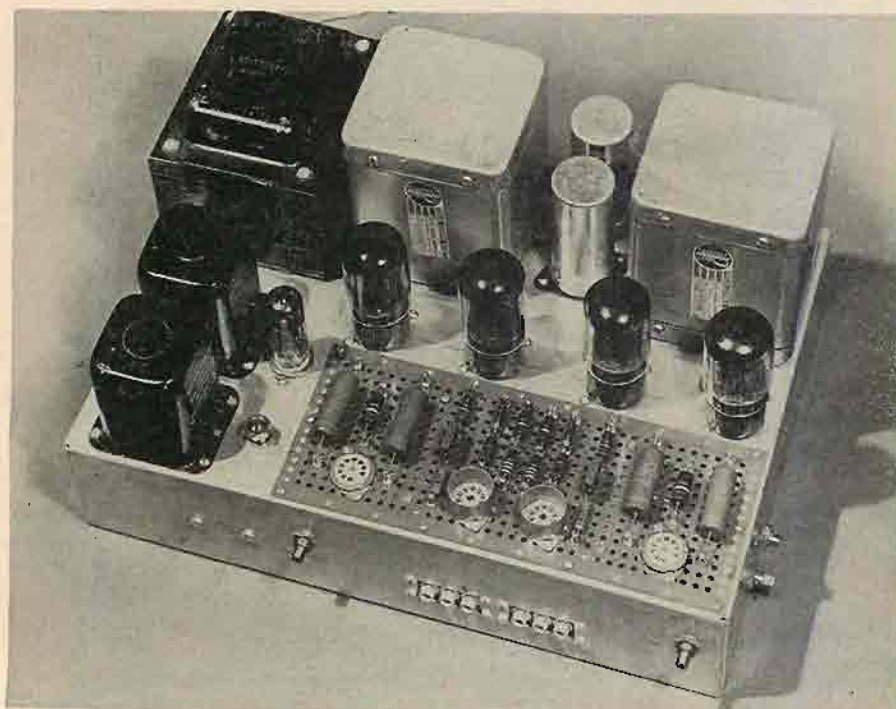
Fig. 1. Top view of amplifier with low-level tubes removed to clarify parts placement on the circuit board.
