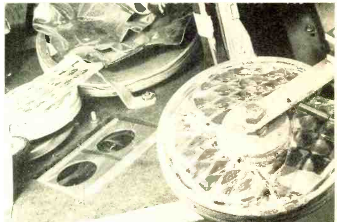
Fig. 20. One of the directly-driven glass-discs has been removed to show the construction. At the left can be seen the two light openings in one of the dual lamp housings, through a hole cut in the Masonite panel.
