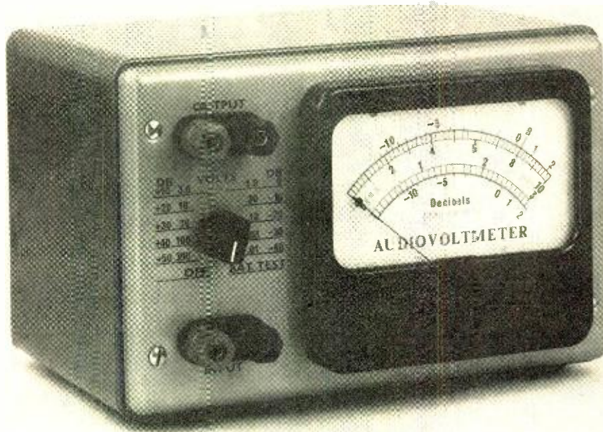
Fig. 1. The completed a.c. voltmeter with ranges from 10 millivolts to 300 volts full scale—and fully transistorized.
