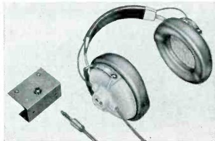
**Specifications:** Dynamic; freq. resp. 20 to 15k cps; impedance 8 ohms; sensitivity 95 db level for 1 mw; plug 3-contact; cord 8 ft.; net weight 10 oz. Price \$29.95. A20-5.
