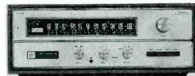
**Specifications:** 4 tubes, 21 transistors, 8 diodes and 2 bridges; golden synchrode front end; 5 i.f. stages; ratio detector; 4 audio stages; meter tuning indicator; output signal 2.0 volts; 5 outputs; controls—tuning, level; switches—power, mode selector, muting; freq. resp.  $\pm$  1 db from 20 to 15k cps; signal-to-noise ratio 70 db; IHF volume sensitivity below noise level; capture ratio 2.0 db; selectivity 55 db; IIF usable sensitivity 1,
