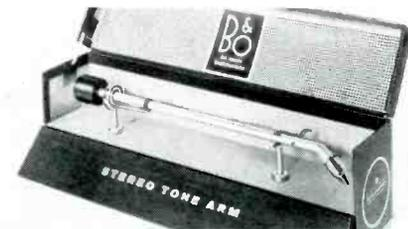
8 $\frac{1}{4}$ "; height range of turntable, 0" to 2"; gimbal suspension; stylus force range 0 to 4 gms; arm material, aluminum; pickup mounting, plug-in; overhang,  $\frac{1}{2}$ "; over-all weight, 1 lb. Price \$49.95. A12-3.
