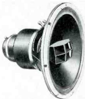
**Specifications:** Type, duplex; power handling capacity, 35 watts; impedance 16 ohms; frequency response, from 20 to 22k cps; magnet weight, l.f. 40 oz., h.f., 8 oz.; voice-coil diameter, l.f. 3", h.f. 1 3/4"; free air resonance frequency 25 cps. Dimensions: 15 5/16" dia., 10" deep; weight, 37 lbs. with network. Price \$168.00. A15-2.
