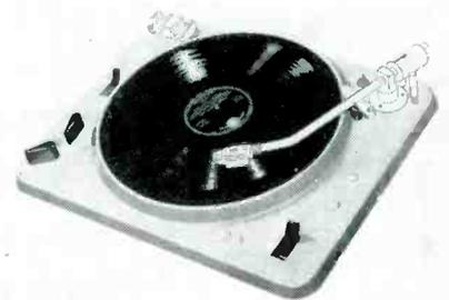
shaft diameter, 1/2"; turntable material, cast iron; felt mat; wow and flutter 0.3% peak-to-peak or 0.1% rms; dimensions of chassis, 15 1/2" x 19 3/4"; clearance required above mounting board, 2"; below, 7"; controls on/off, stereo selector; over-all weight, 22 lbs. Price, \$595.00. Accessories, electronic brake, \$89.50. A13-2.
