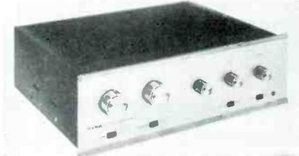
watts per channel; harmonic distortion, 1% at 35 watts  $\pm$  1 db from 20 to 20k cps; IM distortion, 1% at 35 watts; hum and noise, 80 db below 17-watt output; sensitivity, input for rated output—phono, 4 mv, tuner 1 volt; damping factor 10; output impedances 8, 16 ohms; inputs—6 phono, 2 tape head, 2 tape amp, 2 aux, 2 radio; weight, 20 lbs. Dimensions, 13" wide, 4" high, 10" deep. Price \$139.95. Dynaco, Inc. A5-4.
