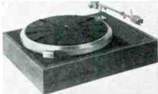
**Specifications:** Speeds—33 1/3 rpm; puck drive; synchronous motor; turntable diameter, 11 27/64"; turntable weight, 2 lb. 7 oz.; shaft diameter, 9/32"; turntable material, alum.; rubber mat; wow, 0.04%; flutter, 0.05%; dimensions of chassis, 14 7/8 x 11 7/8"; clearance required above mounting board, 1 1/2"; below, 3"; controls, on-off; Stanton 400A cartridge; mounting dimensions, 1/2"; number of leads to head, 4; number of cables to chassis, 2. Price, \$129.95. A14-8.
