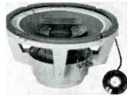
on axis) 0.2 watts; magnet weight—woofer 1 lb. 6 oz.; tweeter 3.16 oz.; voice-coil diameter—woofer 2 1/2", tweeter 1"; free air resonance frequency 50 cps; recommended enclosure volume 3 1/2 cu. ft. min. Dimensions 12 1/4", dia. 7" deep; mounting dimensions, (4) 1/4-in. holes on 11 1/2" circle; cutout diameter 11"; weight, 14 lbs. Price \$70.00. Other features continuously variable high frequency control on 30" cable. A15-5.
