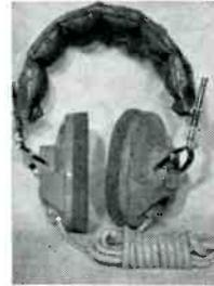
**Specifications:** dynamic; freq. resp. 30 to 15k cps; impedance 8 ohms; maximum power handling 500 mw; plug standard; cord 6 ft.; net weight 11 oz. Price \$11.88. Accessories: F-641 junction box with 2 volume controls. Price \$4.59. A20-8.
