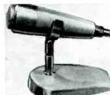
**Specifications:** Dynamic; omni dir. pattern; mylar diaphragm material; die cast case; gray finish; output impedance 2k ohms; freq. resp. +5 db from 35 to 18k cps; sensitivity -55 db; cable connection detachable screw-on standard phone and mini-phone; two lengths of cable furnished each five ft.; chrome slip-on clamp mounting; floor stand coupler also furnished. Price, \$9.95. A19-8.
