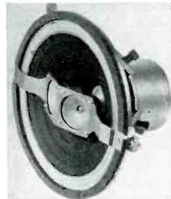
**Specifications:** Type 2-way; power handling capacity 30 watts; impedance 16 ohms; frequency response from 30 to 15,000 cps; magnet weight 29 oz.; free air resonance frequency 40 cps. Price \$79.50. Other features: flux density 12,500 gauss. A15-23.
