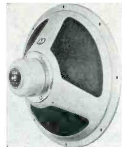
in.; free air resonance frequency 65 cps; recommended enclosure volume 1.5-6 cu. ft. Dimensions: 8" dia., 4" deep; mounting dimensions, 4 holes on RMA std circle; weight 5 lbs. Price \$14.95. A15-15.
