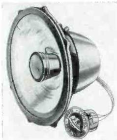
frequency response, from 30 to 15k cps; magnet weight 20 oz.; free air resonance frequency 40 cps; recommended enclosure volume 6 cu. ft. Dimensions: 12 $\frac{1}{2}$ " dia. 6 $\frac{1}{8}$ " deep; cutout diameter 10 $\frac{1}{2}$ "; weight 11 lbs. Price \$29.50. Other features: brilliance level control. A15-11.
