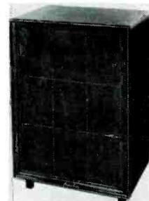
*Specifications:* dual phase inverter enclosure; speakers—12" l.f., 8" h.f.; power handling capacity 40 watts of organ tone; 300 cps 1/4-section crossover network; impedance 8-16 ohms; frequency response ± 5 db from 32 to 13k cps; magnet weights: l.f., 22 oz.; h.f., 12 oz.; voice-coil diameters: l.f., 2"; h.f., 2". Dimensions: 24" wide, 36" high, 19" deep; weight, 80 lb.; standard walnut \$150.00; unfinished birch \$125.00; to specification \$165.00. A16-16.
