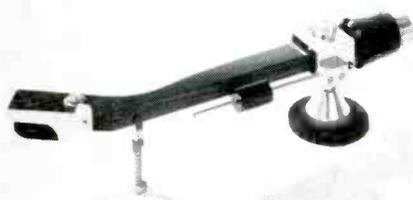
nut; pickup mounting, standard on slide; overhang,  $\frac{3}{8}$ "; maximum tracking error,  $\pm 0.5$  deg; additional features, stylus overhang adjustable, interchangeable cartridge slides; arm resonance—11 cps. Price \$45.00; extra cartridge slides, \$2.95. A12-5.
