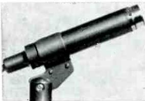
**Specifications:** condenser; omni dir. pattern; vac. plated alum. alloy diaphragm material; alum. and stainless steel case; enam. finish; output impedance 200 ohms; freq. resp. +3 db from 20 to 20k cps; sensitivity -52 db; cable connection cannon XL; length of cable furnished 20 ft.; cannon plug; dimensions—7/8" x 5"; weight 4 1/2 lbs; standard 5/8" swivel mounting. Low Z, price \$150.00. High Z, price, \$130.00. A19-13.
