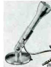
output impedance 250k ohms; freq. resp. 50 to 10k cps; sensitivity -58 db; length of cable furnished 7 ft.; phone plug; dimensions—1 9/16" dia., 5 1/4" long; weight 0.4 lbs; hand held unaffected by heat or moisture. Price, \$18.50. Accessories: CMS-10 stand (die-cast). Price, \$5.00. A19-19.
