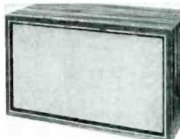
crossover networks; impedance 8 ohms; frequency response 30 to 30k cps; magnet weights: l.f., 16 oz.; finished on 4 sides. Dimensions: 24" wide, 14" high, 12" deep; weight, 30 lbs.; oiled walnut veneer \$79.95. A17-24.
