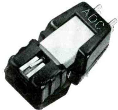
recommended tracking force—professional arms, 0.75–1.5 gms; compliance—lateral, 30  $\times$  10<sup>-6</sup> cm/dyne, vertical, 30  $\times$  10<sup>-6</sup> cm/dyne; inductance, 500 mh; d.c. resistance, 700 ohms; 4 terminals; mounting dimensions, 7/16" or 1/2". Price, diamond, \$60.00; replacement styli, elliptical—\$25.00; regular—\$15.00. A11-1.
