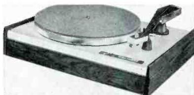
**Specifications:** Speeds—33 1/3 rpm; direct rim drive; 12-pole synchronous motor; turntable diameter, 12"; turntable weight, 12 oz.; shaft diameter, 1/4"; turntable material, aluminum; foam mat; wow, 0.03%; flutter 0.04%; dimensions of chassis, 17" x 14"; clearance required above mounting board, 3"; below, 2"; type of mounting, walnut base included; controls, on-off; over-all weight, 12 lbs. Price, \$59.95. A14-10.
