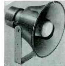
Specifications: horn; power handling capacity 30 watts; impedance 8 ohms; frequency response, 250 to 15k cps; Dimensions 9¾" dia. 8 13/16" deep; shpg. weight, 8½ lbs. Price \$16.50. CS4-5.
