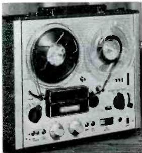
ips, ± 5 db from 60 to 14k cps; 5/16 ips. ± 5 db from 80 to 4k cps; signal-to-noise ratio, 40 db; wow and flutter, ± 3% at 7 1/2 ips, rewind time, 96 sec. Inputs—1 microphone. Dimensions, 12" wide, 10 1/4" high, 5 1/4" deep; weight, 12 lbs. Tape counter, pause, built-in power supply. Price \$199.95. Accessories: stop-start foot control \$4.95. A18-19.
