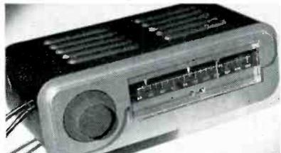
freq. resp.  $\pm 1$  db from 50 to 15k cps; AM suppression 35 db; harmonic distortion (100% mod.) 1%; stereo separation 35 db; switching stereo circuit; reactance tube a.f.c. circuit; drift 15 kc; dimensions: 10 1/2" wide, 3 3/4" high, 8" deep; weight, 9 lbs. Price \$94.00. A7-15.
