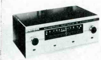
**Specifications:** 12 tubes; cascode front end; horiz. bar tuning indicator; controls—tuning; switches—power, a.f.c. defeat, muting, mpx noise filter, stereo-mono; freq. resp.  $\pm$  1 db from 20 to 20k cps; sensitivity 1.2  $\mu$ v for 20-db quieting with 300 ohm antenna; stereo separation 30 db; time division stereo circuit; dimensions: 15" wide, 5 1/2" high, 11 1/8" deep; weight, 12 1/4 lbs. Price \$359.00. A7-1.
