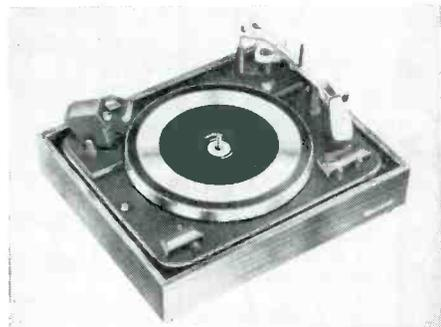
ribbed with chrome insert mat; dimensions of chassis, 16¾" x 14½"; clearance required above mounting board, 6"; below, 2¾"; type of mounting, barrel springs; controls, manual and auto on/off; automatic cycling time, 10 secs at 33½ rpm, 3½ sec at 78 rps; type of pickup head, plug-in 4 pin; material, plastic;
