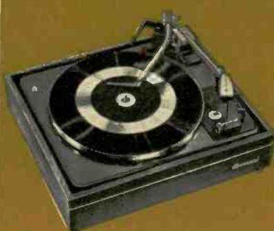
**AT60** An automatic turntable with intermix capabilities. Meets all the critical performance standards required of a Garrard Automatic Turntable, plus compact versatility. Four speeds. Features tubular tone arm, dynamically balanced and counterweight adjusted; built-in stylus pressure gauge; heavy, oversized, die-cast, non-magnetic turntable; Laboratory Series® motor. **\$59.50**
