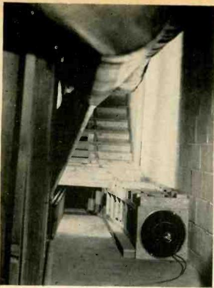
Fig. 2. The throat end of the horn, showing the 15-in. driver.
