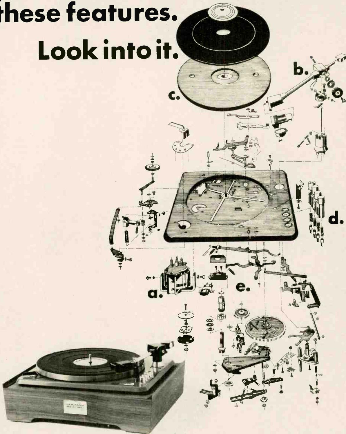
**a.** Hysteresis Motor. The 40H is the only automatic so equipped. Maintains accurate speed even with extreme voltage variations. Uses famous Papst motor, found in professional turntables and tape transports.
