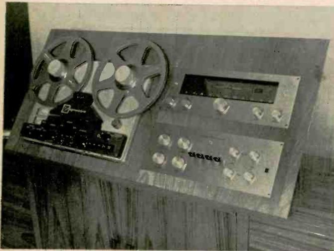
Close up of the control panel which accommodates the tape recorder, tuner, and preamp.
