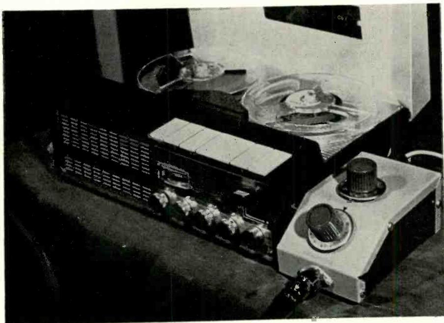
Fig. 1. Converted Uher 4000 Report-S, with output coupling unit/microphone pre-amp at the right.
