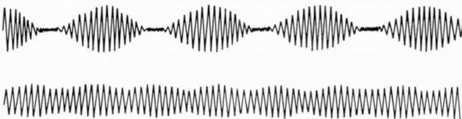
Fig. 1. A special waveform consisting of a signal of frequency,  $f$ ,  $f + f_1$  and  $f - f_1$ . The phase of the two sidebands can be adjusted to give an amplitude-modulated signal above or a smoother frequency-modulated signal below.
