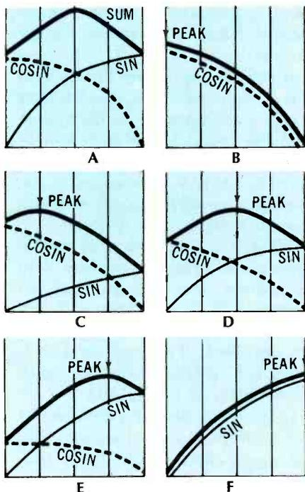
Fig. 6. Continuing the development of the sine-cosine theory, where the summation is shown at A, with the remaining figures showing the sound distribution over the separate speakers.
