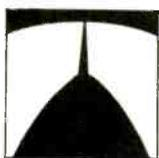
But as the head begins to wear down, the pole gap widens, causing frequency response to decline. To maintain original frequency response, heads may need replacement after as little as 500 to 1000 hours of normal playing.
