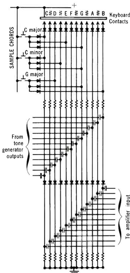
Fig. 7-6—Using diodes for coupling notes played by chord buttons.
