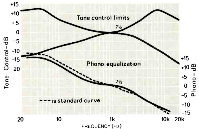
Fig. 6. Curves of tone-control action and the pickup input equalization.
