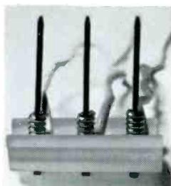
**"Wire-wrap" — a permanent connection technique that eliminates solder joints:**
