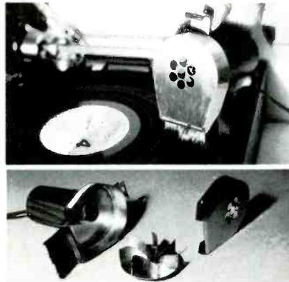
Then I reversed the procedure, and made a blower with a soft brush attachment. You hold it over the spinning record for a few seconds and it blows the finest dust off without leaving any magnetic static.
