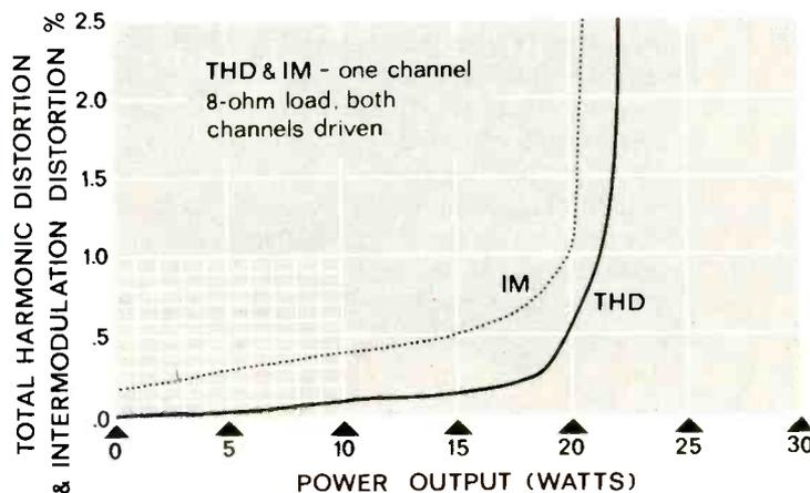
Fig. 1 — Typical power output vs. Total Harmonic Distortion curve for an amplifier. To conserve space, the corresponding Intermodulation Distortion curve is shown on the same graph.
