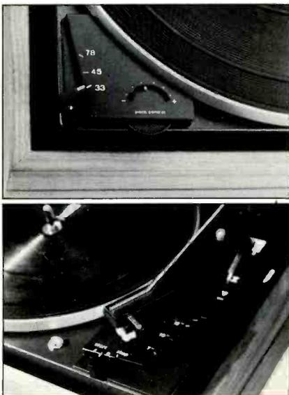
At the left front of the motor board is the speed selector, a plastic lever; adjacent to it is a knurled flat knob which is the vernier speed control, protected by a sliding plastic guard so that once set, it is not likely to be moved accidentally.
