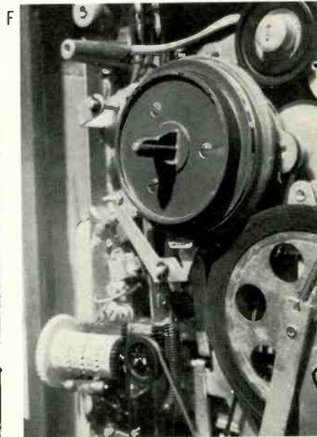
(F) Examples of the wide, thin take-up idler on a loose bracket which is liable to misalignment, and the smaller soft-tired auxiliary wheel at right. Philips 3548.
