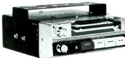
Power requirements are 12 volts (auto battery, positive or negative ground). Signal-to-noise ratio is 45 dB; wow and flutter, 0.28% 1% ips; outputs, two extension speakers (impedance for each channel is 3.2 ohms). Dimensions are 2 7/8" H x 7-3/16" W x 8 1/4" D. Price is under \$119.50, complete with car mounting bracket and hardware, head-cleaning device, and a coupon for purchase of a 3-pack of prerecorded Superscope cassette albums at a special introductory price of \$8.85.
