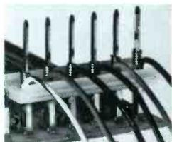
"Wire-Wrap" . . . a permanent connection technique that eliminates solder joints.
