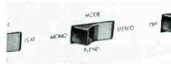
Center channel speaker can be driven without an auxiliary amplifier with mode switch in BLEND, which also reduces unrealistic stereo separation when using headphones.
