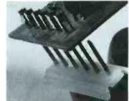
Snap-in printed circuit modular construction for reliability and ease of service.
