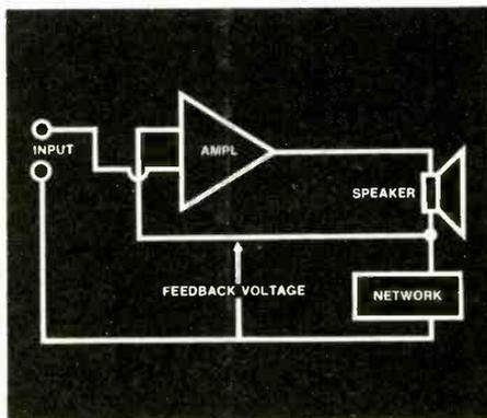
The above circuit illustration shows how feedback voltage is derived when the LWE is connected to amplifier. A voltage is developed and fed back to the same point in the amplifier that the negative voltage feedback enters.
