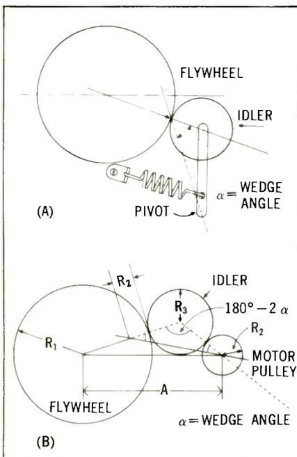
Fig. 1—(A) Wedge angle is important for correct transmission of torque. (B) Distances and wedge angles can be calculated when diameters of motor pulley and flywheel are known.
