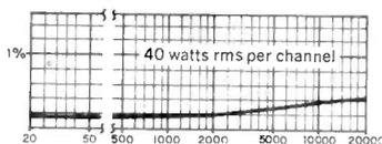
The SCA-80 delivers 40 watts per channel rms continuous power from 20-20,000 Hz at 8 ohms. Plenty of power for driving 4 ohm speakers too.
