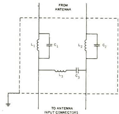
Circuits tuned to interfering signal.
