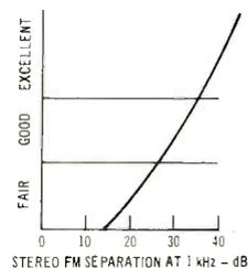
Fig. 4—Stereo FM separation at mid-frequencies
