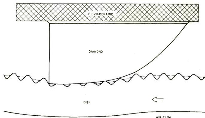
Fig. 3—Showing the shape of the stylus and the way it can glide over the grooves
