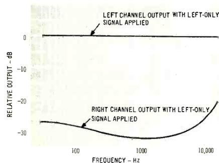
Fig. 6—Typical stereo separation curve
