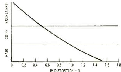
Fig. 9—Ratings for IM distortion
