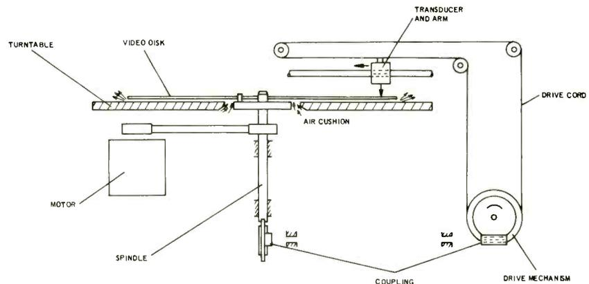
Fig. 2—The turntable drive system
