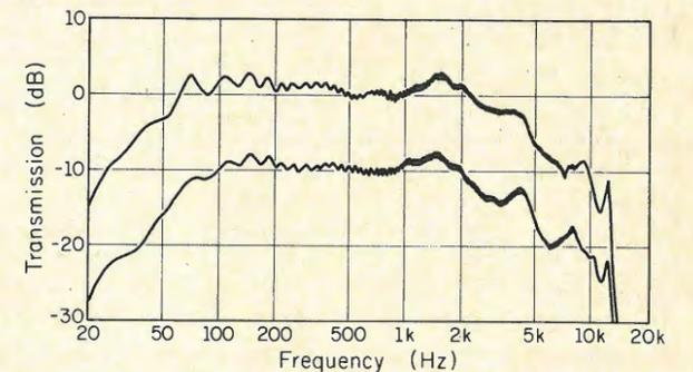
Fig. 9—Effect of the R-70 cavity. The upper-curve response is for the same conditions as in Fig. 8, except for the added 0.22-inch cavity in front of the R-70 pickup. The lower curve is for a duplicate tube made to the same mechanical specifications and using other specimens of the same transducers. The 10 dB displacement is a plotting artifact.
