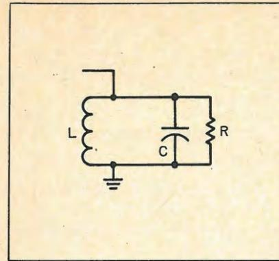
Fig. 2—Equivalent circuit of any parallel resonant tuned circuit. The frequency of resonance is determined by values of "L" and "C" while "Q" is a function of the equivalent resistance of "R."
