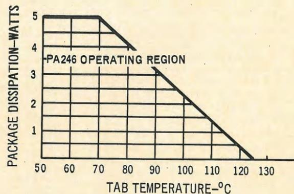
Fig. 8—Allowable PA246 package dissipation as determined by measured tab temperature.
