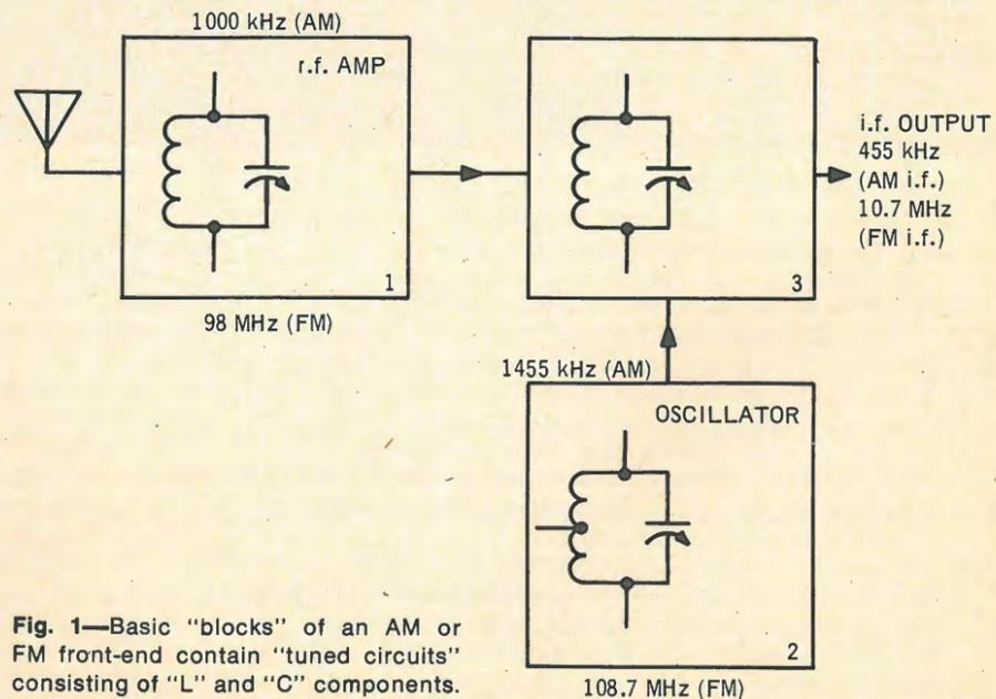
Fig. 1—Basic "blocks" of an AM or FM front-end contain "tuned circuits" consisting of "L" and "C" components.
