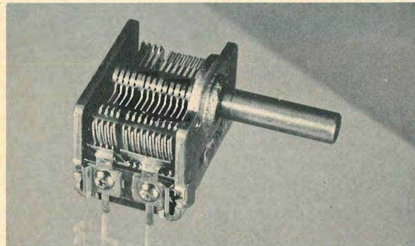
Fig. 3—An AM variable tuning capacitor.
