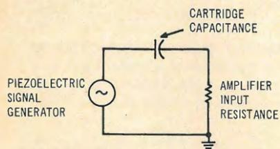
Fig. 1—Equivalent circuit of piezoelectric cartridge and load resistance.
