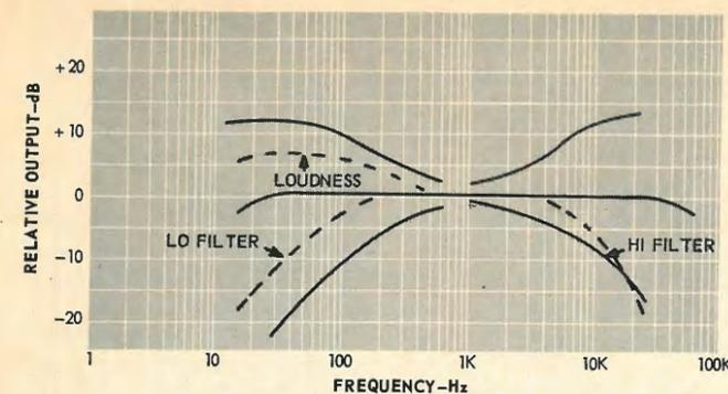
Fig. 7—Frequency response, tone control range, filter characteristics, and loudness control response (at -30 dB).
