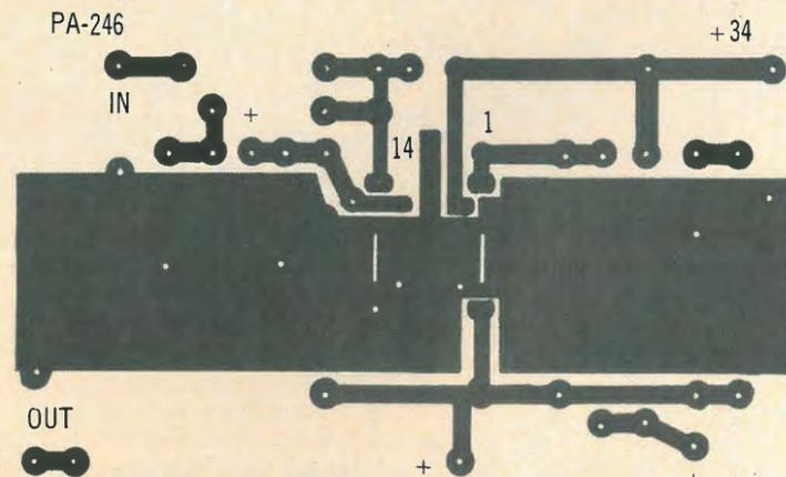
Fig. 10B—Pattern for printed circuit side of board.
