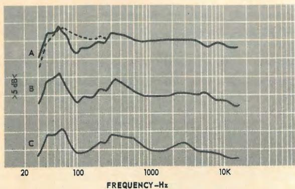
Fig. 2—Frequency response, (A) on-axis, (B) 45 degrees off-axis, and (C) average of six curves at different points about the speaker's axis.
