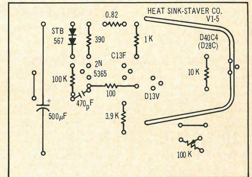
Fig. 13A—Parts layout for the component side of the PC board.
