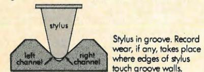
As the record rotates, the rapidly changing contours of both groove walls force the stylus to move up, down and sideways at great speeds.
