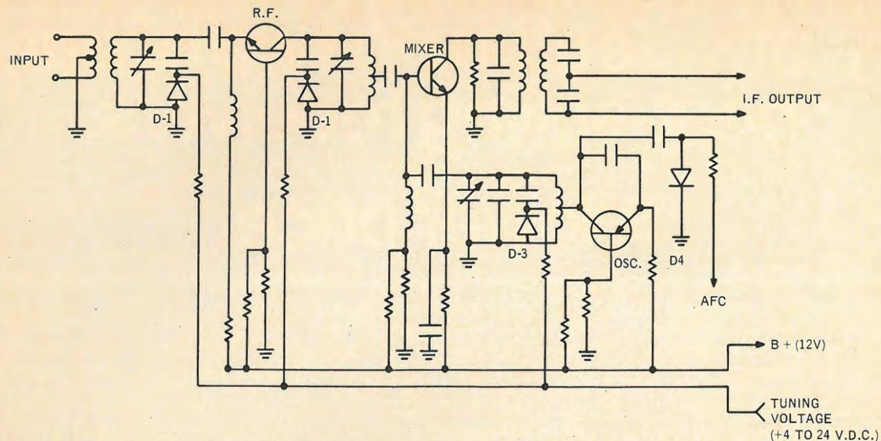
Fig. 7—Basic FM front-end by Görler, using three varactor diodes instead of the usual variable capacitor.
