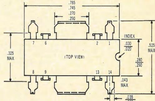
Fig. 6—Five watt IC package and outline giving lead identification.
