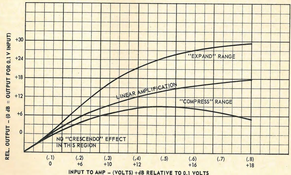
**Fig. 2—Range of crescendo control in expand and compress modes.**
