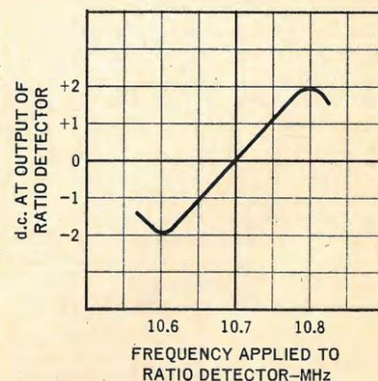
Fig. 6—Varying d.c. voltage at the output of the FM detector is used to automatically correct for improper tuning of stations.
