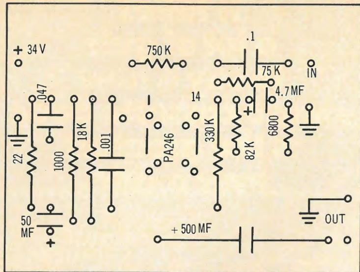
Fig. 10A—Parts layout, component side of PC board.
