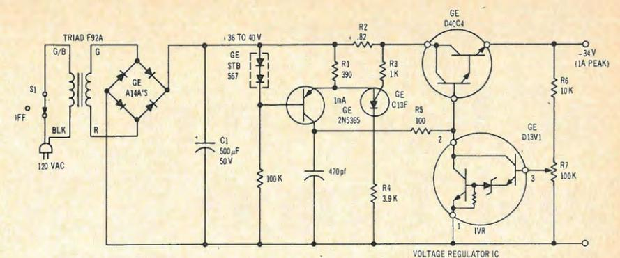
Fig. 12—Regulated power supply with electronic circuit breaker protection.
