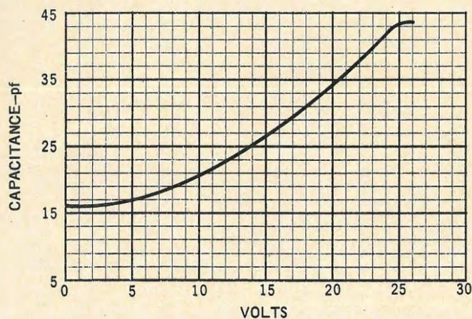
Fig. 8—Change in capacitance with applied voltage of a typical varactor diode.
