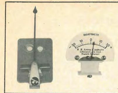
Fig. 1—Moving element of the magnetometer consists of a small disc magnet (seen under the horizontal vane) and the pointer, all mounted in the brass fixture with adjustable bearings.
