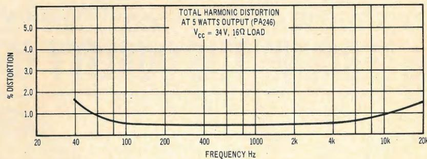
Fig. 5—Distortion versus frequency for PA246.
