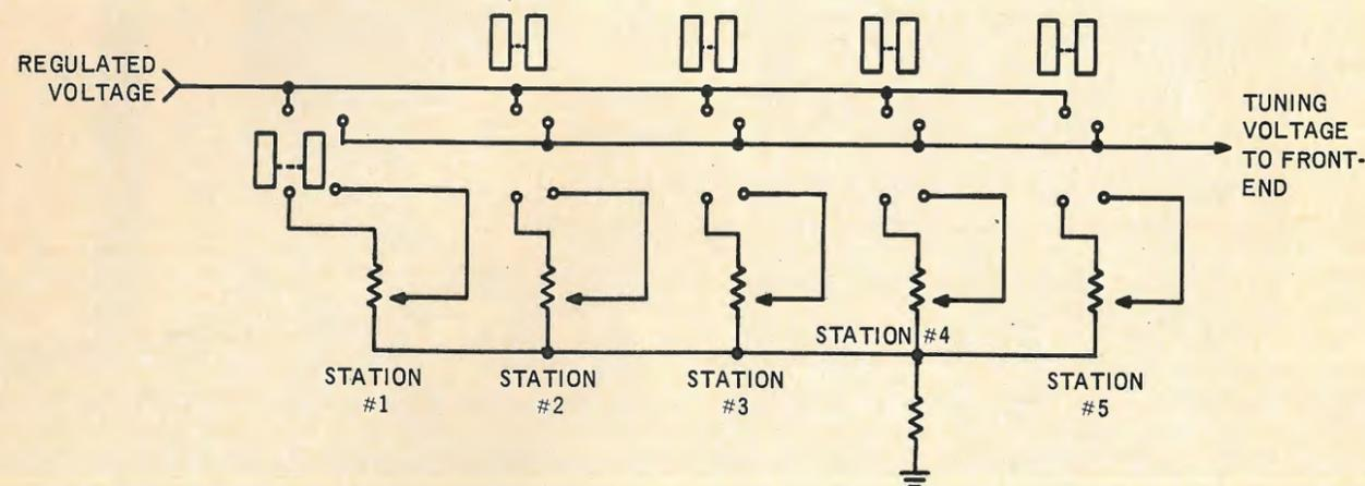
Fig. 11—Five individual potentiometers, singly selected by pushbuttons, tune the varactor-diode front-end to preselected station frequencies.
