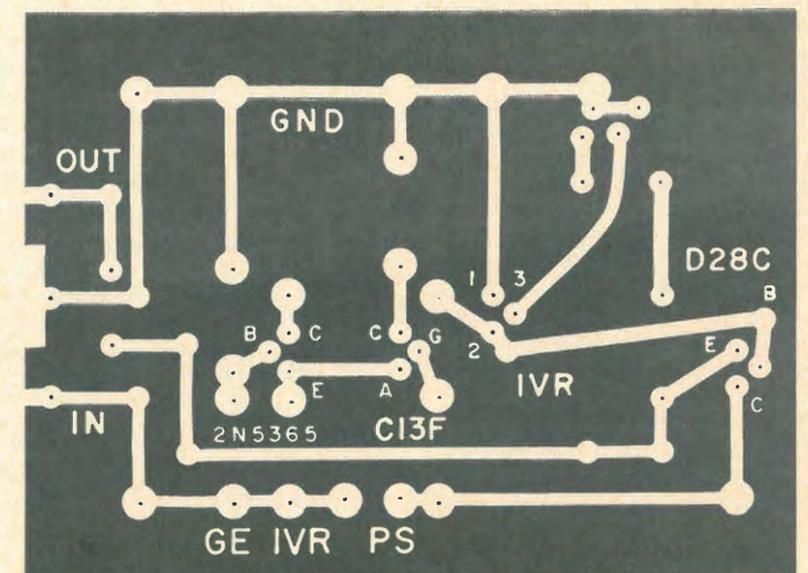
Fig. 13B—Pattern for the printed circuit side of the board.
