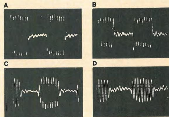
Fig. 3—Toneburst response at (A) 500 Hz, (B) 1000 Hz, (C) 5000 Hz, and (D) 10,000 Hz.
