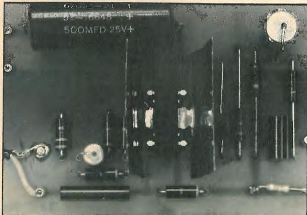
Fig. 7—Complete circuit assembly of five watt IC assembly diagramed in Fig. 3.
