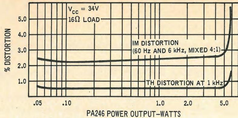
Fig. 4—Typical distortion versus power output level for PA246.
