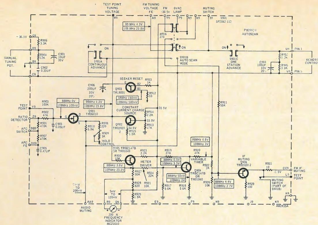
Fig. 12—Complete circuit diagram of Fisher Radio's "Autoscan" as used in the Model 450-T.
