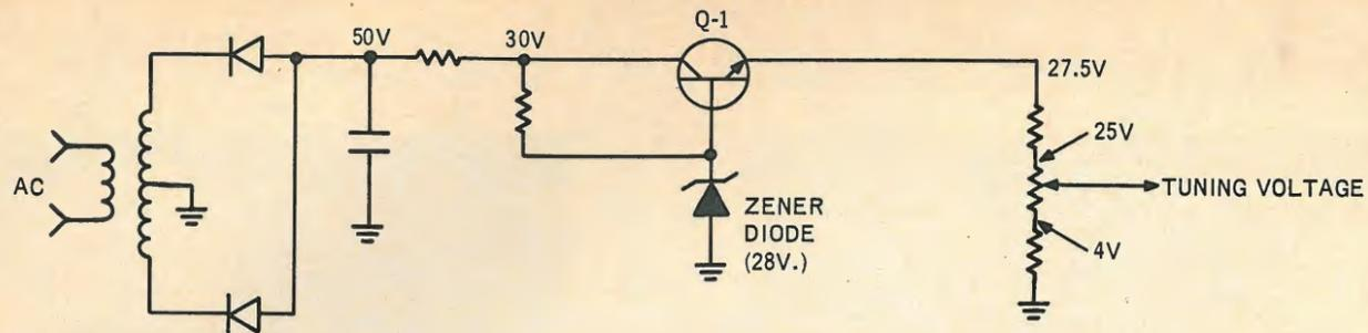
Fig. 10—A Zener-diode regulated power supply provides tuning voltage. Transistor Q-1 improves temperature stability of the system.
