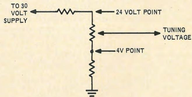
Fig. 9—A potentiometer acting as a voltage divider could easily serve as the "tuning control" for the circuit of Fig. 8.
