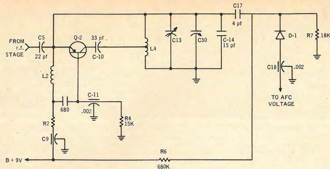
Fig. 5—Converter stage utilizing a regular variable capacitor, as well as fixed values of "C" to tune the local oscillator.
