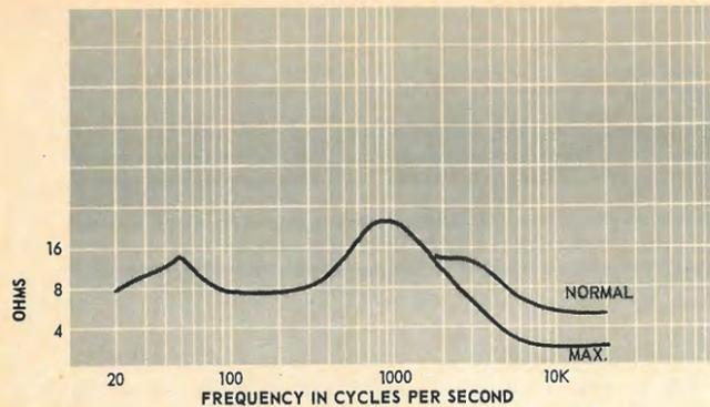
Fig. 1—Impedance of the AR-2ax with tweeter level controls at normal and maximum positions.
