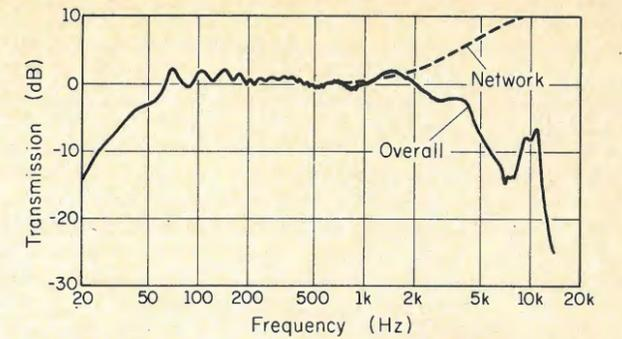
Fig. 8—Equalization obtained with the R-50 collar and cavity and passive networks. The setup used coiled tubing. The two passive networks embodied in the overall response has the joint response shown in the dashed curve.
