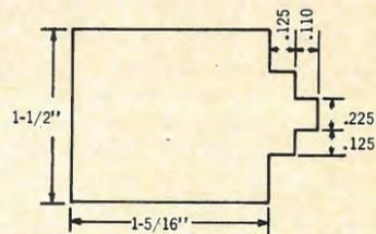
Fig. 9—Heat radiating fin of 0.015" copper.
