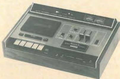
mode it was set for, yet without the tape movement. There are 36 transistors and 30 diodes in the device, and two microphone jacks on the front panel accommodate dynamic mics. Line input and output phono jacks are located on the rear of the walnut-finished cabinet. There are two erase heads—each covering its half of the tape—and one four-track record/play head. The synchronous drive motor
