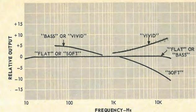
Fig. 8—Response in fixed "tone setting" positions.
