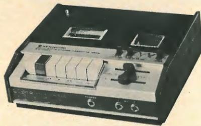
of the unit is equipped with a line-voltage switch, allowing use with supplies from 100 to 240 volts; as well as with a fuse, two phono jacks for line input, two more for line output, and a DIN receptacle for connection with receivers or amplifiers so equipped, using a single cable. The front apron accommodates a headphone jack for use with conventional 8-16 ohm phones, a pair of phone jacks for microphone inputs. Frequency response is within
