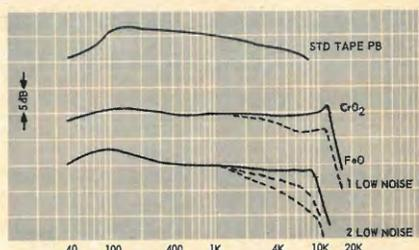
$\pm 2$  dB from 40 to 12,000 Hz with CrO<sub>2</sub> tape and within  $\pm 3$  dB from 40 to 9500 Hz with FeO tape. The hi-filter droops response about 4 dB at 10 kHz with CrO<sub>2</sub> tapes, and the curves for FeO tape show the effect of using the hi-filter during both recording and playback modes, showing a droop of 8 dB compared to the 4-dB droop when used in only the playback mode.
