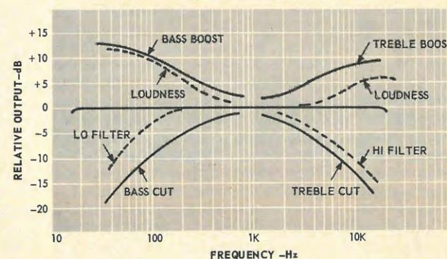
Fig. 9—Frequency response, tone, loudness, and filter characteristics.
