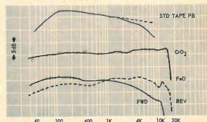
held speed within -2.5 per cent at 85 volts to +0.6 per cent at 135. Frequency response with CrO<sub>2</sub> tape was within  $\pm 2$  dB from 40 to 14,000 Hz in the forward direction, slightly less in the reverse direction. With FeO tape, response was about the same, extending only to 12,000 Hz. With the limiter switch on, response at 10 kHz was down an additional 6 dB.
