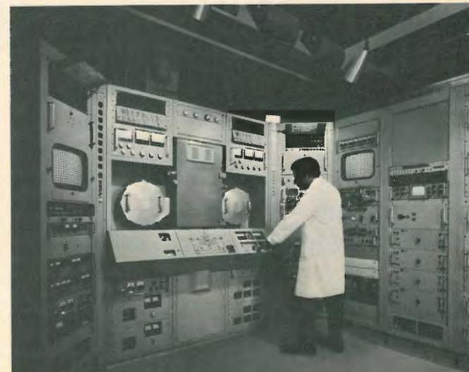
Fig. 3—The electron beam recorder.
