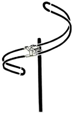
Fig. 1—The Channel Master 4405 antenna is a folded dipole bent into an "S shape."
