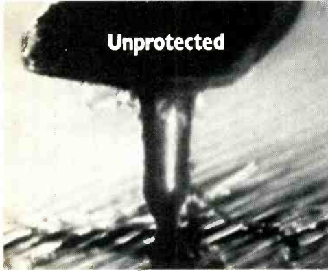
Magnification shows the record vinyl wearing away.
