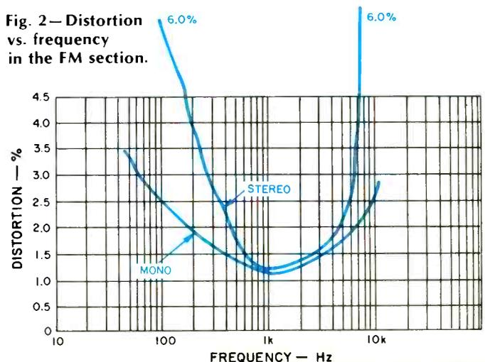
$\mu\text{V}$  (20.8 dBf). Since the AFC circuitry of this tuner section is always operative, it was impossible to determine selectivity characteristics accurately, but in our listening tests we found it pretty difficult to separate closely spaced weak and strong signals, since the tuner always "homed in" on the stronger station. From the point of view of the city driver, this is a benefit rather than a negative characteristic, as it does tend to keep the signal locked in.
