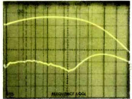
corresponds to 3.42 watts. The 10 per cent total harmonic distortion point occurred with a power output of 4.62 watts, lower than the 6 watts per channel claimed by the manufacturer.
