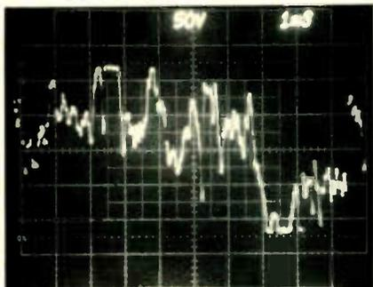
**Fig. 2—Peak-to-peak voltage in bridged mono mode measured 240 V under actual music signal conditions.**
