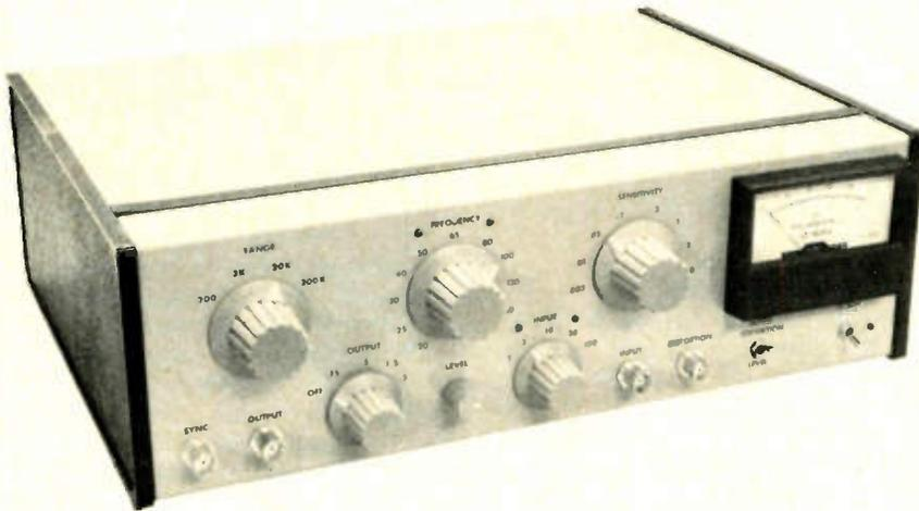
Fig. 3 — Exterior view of the completed THD analyzer.
