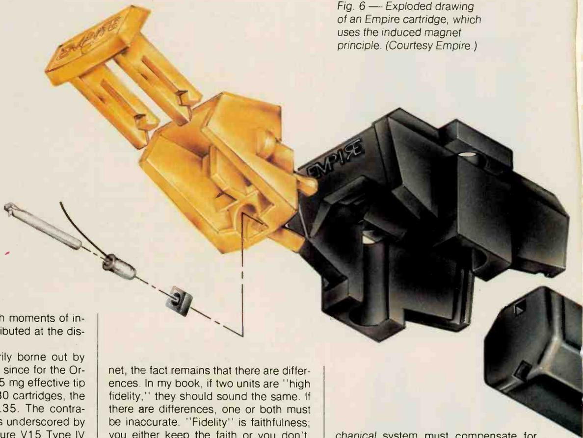
Fig. 6 — Exploded drawing of an Empire cartridge, which uses the induced magnet principle. (Courtesy Empire.)
