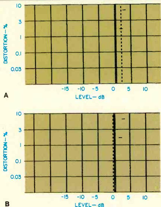
**Fig. 5 — A slight improvement in 3rd-order harmonic distortion was noted when 16-bit mode is used on Sony PCM-F1 (A), but so long as recording level does not exceed 0-dB (B), 3rd-order HD is insignificant in both 14- and 16-bit modes.**
