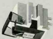
**DL-301** To control resonances, the cantilever fulcrum of all Denon MC cartridges is independent of the damping rings. The DL-301 uses two damping rings, each optimized for its portion of the frequency range.
