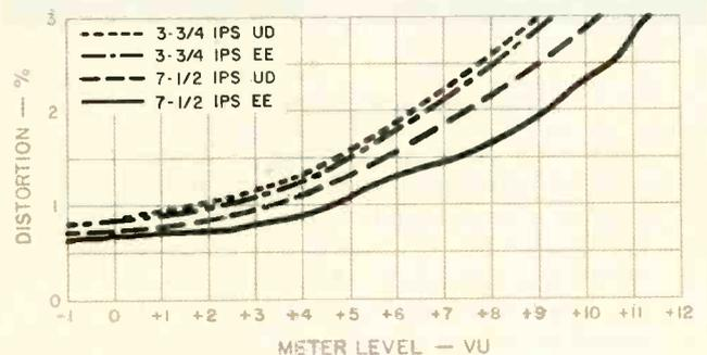
**Fig. 3 — Distortion and headroom at 1 kHz.**
