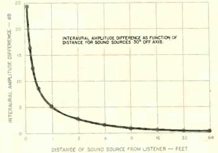
Fig. 1A—Interaural amplitude differences diminish rapidly with increases in distance from the sound source.
