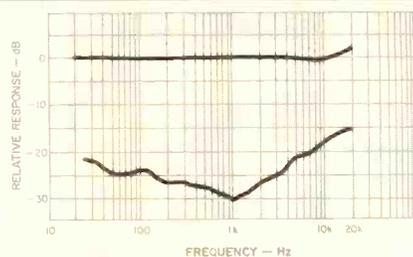
Fig. 1 — Frequency response and separation.
