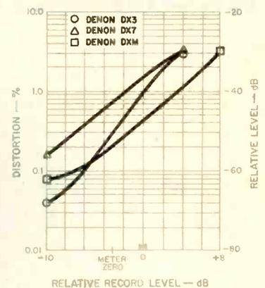
Fig. 5—Third harmonic distortion vs. level in Dolby mode at 1 kHz with Denon DX3, DX7 and DXM tapes.
