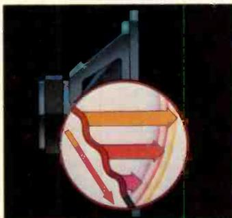
Ohm Walsh 2™ loudspeaker — single arrow represents pulse travelling down inverted surface causing in-sync fragments (as represented by 3 horizontal arrows) to enter air along the way eliminating the problem of stereo ghosts.
