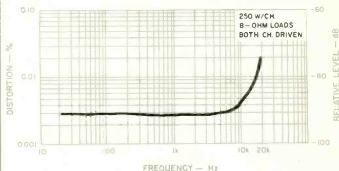
Fig. 2—THD vs. frequency at rated output.
