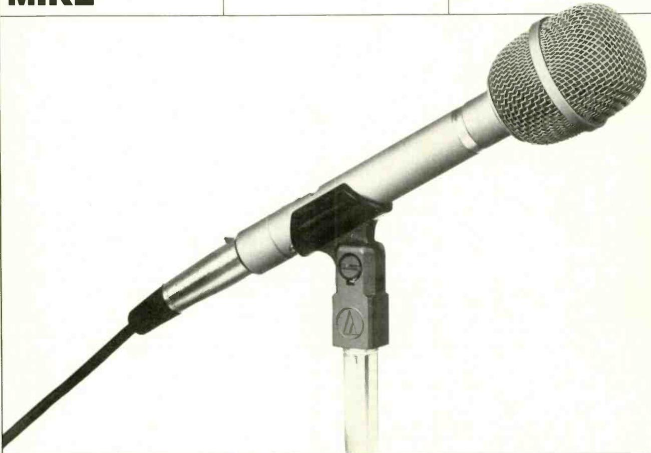
The Audio-Technica Model AT813 is a cardioid unidirectional electret microphone powered by an internal battery. It was designed for audiophile or professional recording applications, or sound reinforcement. The large metal screen on the head end encloses an integral wind/pop screen. The
