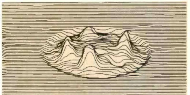
**Fig. 6B**—A high-resolution plot at 14,274 Hz shows a severe, four-pole bell mode.
