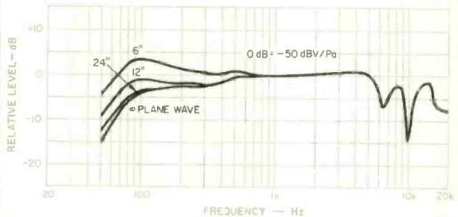
Fig. 5—Frequency response vs. distance from source (sample #1).
