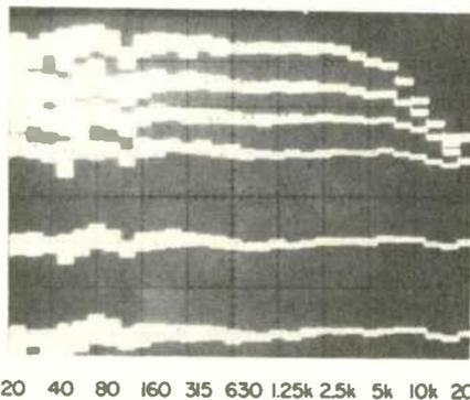
**Fig. 5—Spectrum analysis of pink-noise response at +14, +8, +4, 0, -10 and -20 dB recording level.**
