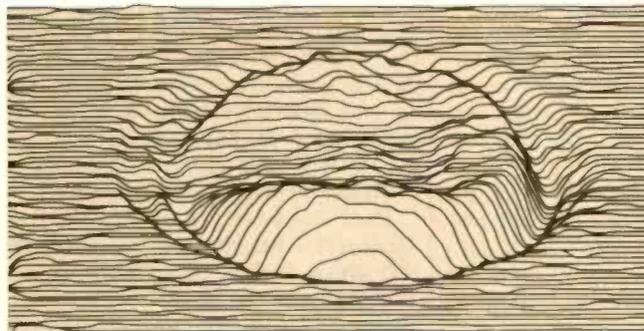
**Fig. 5B**—At 1022 Hz, laser-computer animation reveals a rocking mode, caused by the mass of the lead-in wires.
