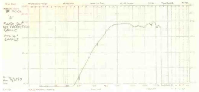
**Fig. 6A**—Sharp 14- and 21-kHz dips mark amplitude response of a 3/4-in. Mylar tweeter, which is relatively flat from 1.1 to 28 kHz.
