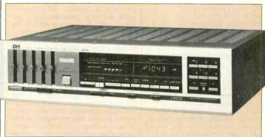
*Instead of conventional tone controls the JVC R-X40 has a five-band graphic equalizer.*
