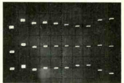
Fig. 2—"Tape recorder" response before (top) and after (middle) equalization, with actual equalization (bottom). (Vertical scale: 10 dB/div.)
