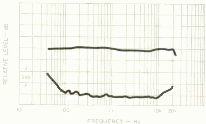
**Fig. 2—Frequency response and separation.**
