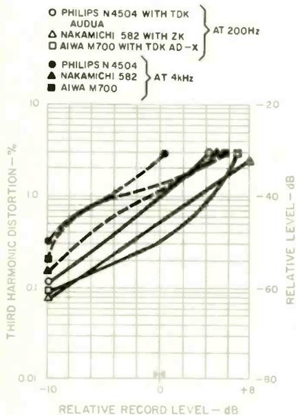
Fig. 7—HDL<sub>3</sub> vs. recording level at 200 Hz and 4 kHz for three recorder-tape combinations.
