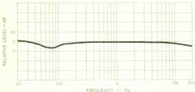
**Fig. 2—Frequency response loss due to loading of our microphone preamp.**
