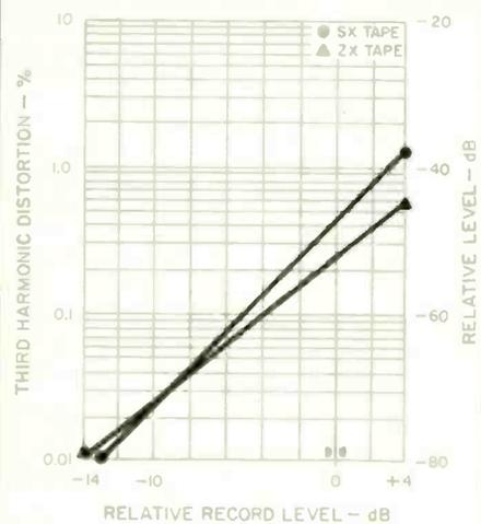
Fig. 6—HDL<sub>3</sub> as a function of recording level at 1 kHz with Nakamichi SX and ZX tapes on 700ZXL recorder.
