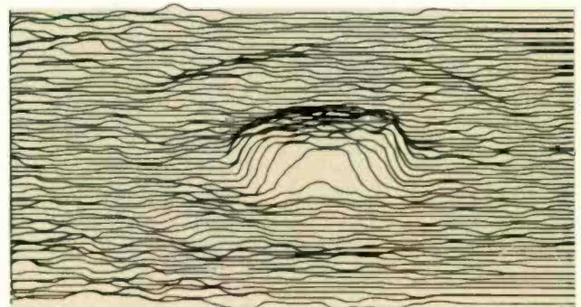
**Fig. 4—A severe dust-dome problem shows up in the bass/mid unit at 1.3 kHz.**
