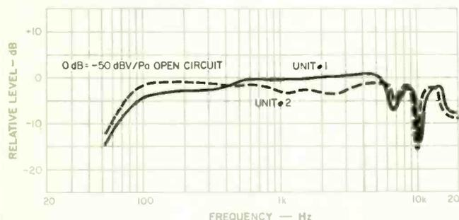
**Fig. 3—Plane wave frequency responses for two AT813 samples.**
