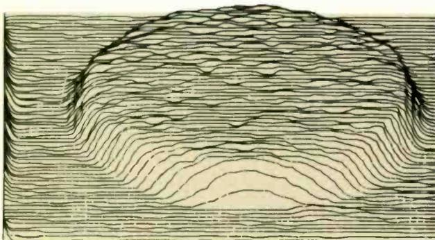
**Fig. 2C—Copper alloy treble unit at 8 kHz is correctly controlled, nearly a perfect piston.**
