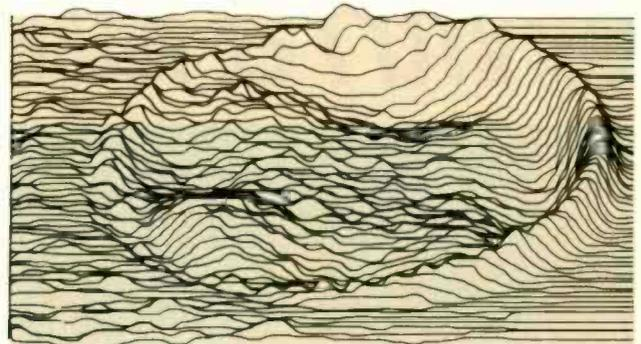
**Fig. 3—At 780 Hz., this conventional bass/mid-range unit shows four irregular bell modes and an asymmetric surround problem.**
