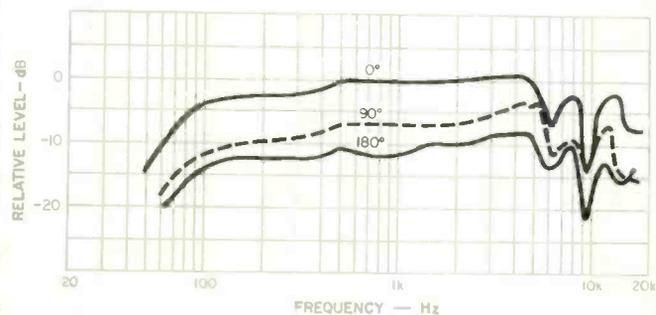
Fig. 6—Frequency response vs. angle (sample #1).
