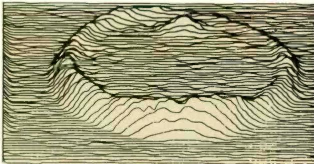
**Fig. 2B—Ultra hard metal dome shows asymmetric decoupling of its surround at 8kHz.**
