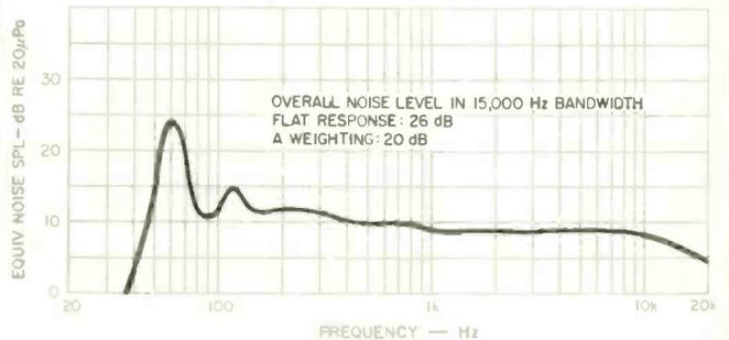
Fig. 7—Microphone noise spectrum (one-third octave bands) of AT813.
