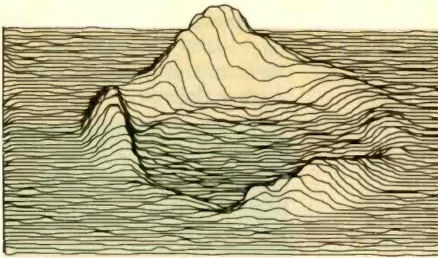
**Fig. 2A—At 8kHz, this 19mm plastic-dome tweeter shows severe asymmetric surround resonance.**
