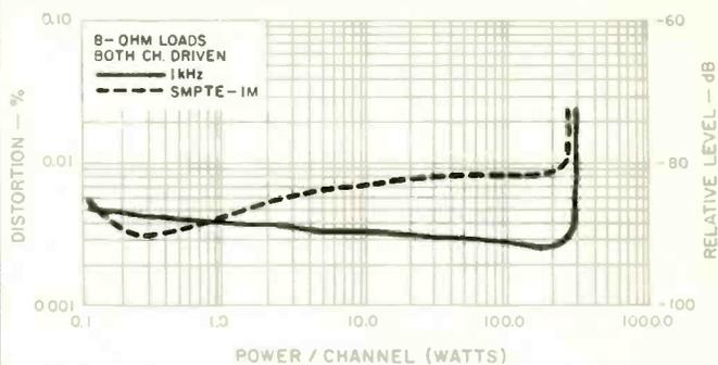
Fig. 1—Distortion vs power output, Heath AA-1800 power amplifier.
