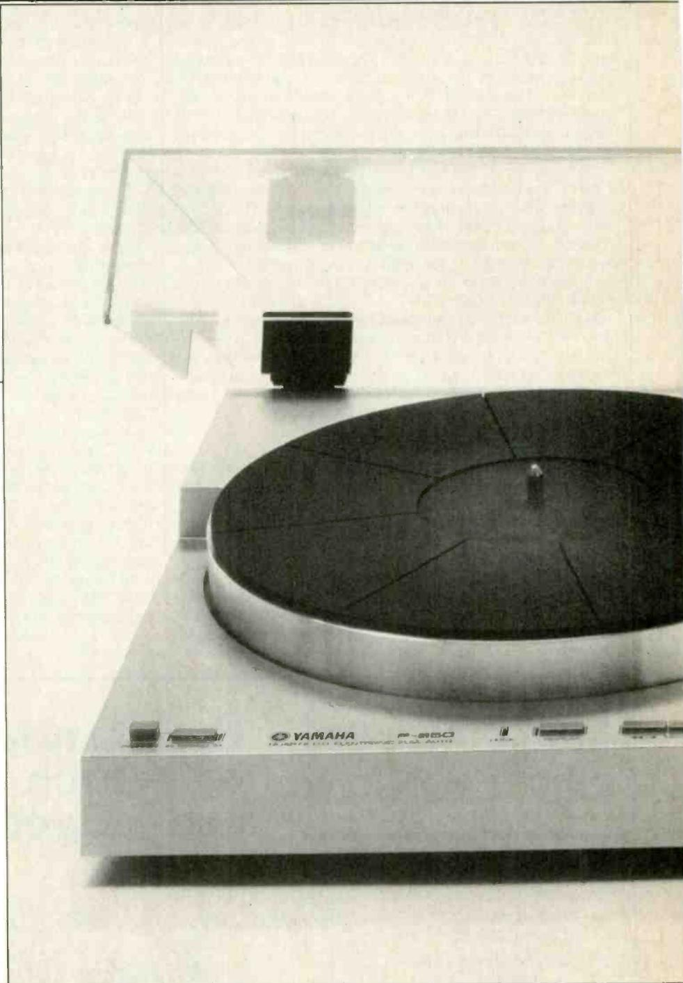
Yamaha's new P-850 is a typical example of modern turntable design, with its sleek, low-profile styling and impeccable performance. It uses a direct-drive servo-controlled motor, while its arm is controlled by two separate motors. The arm itself is a straight tubular type, mounted on a platform at the rear, which extends the full width of the unit. A neat rectangular counterweight slides on two run-
