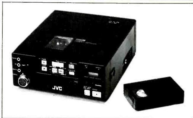
tery pack, the VCR weighs only 4.4 pounds; with the battery pack, it tips the scale at just 5.3 pounds. The TC-20 videocassette is about the size of a deck of playing cards.
