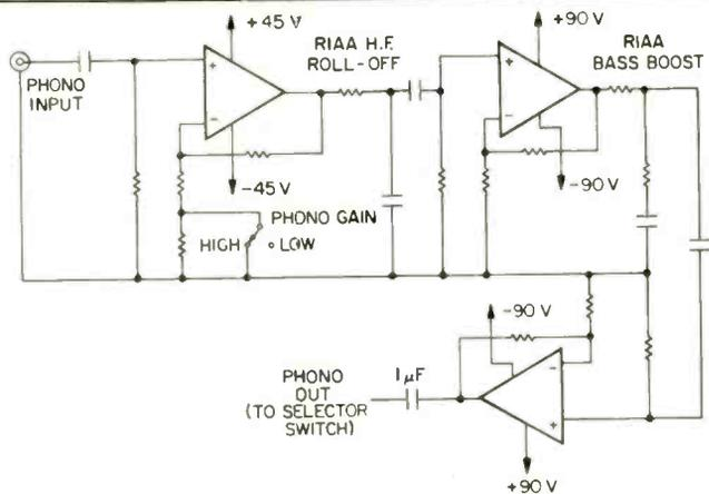
Fig. 1—Phono-circuit block diagram.
