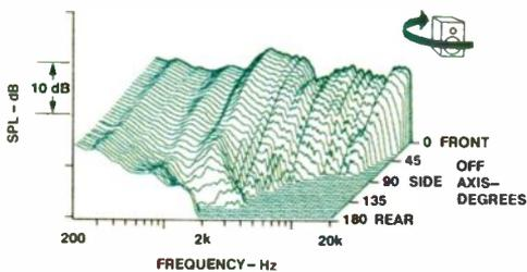
**Fig. 3—Horizontal off-axis frequency responses.**
