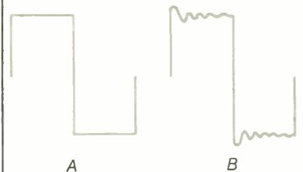
Fig. 2—Square wave before (A) and after (B) phase shift.
