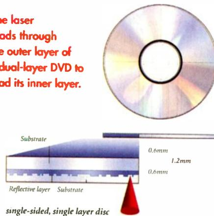
A semi-transmissive film and a dual-focus laser system enable two data layers to be read on a single side!
