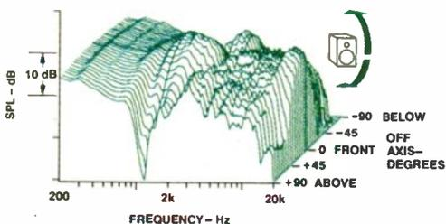
**Fig. 4—Vertical off-axis frequency responses.**
