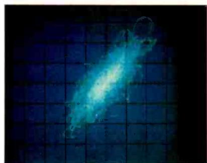
Fig. B2—Lissajous pattern showing (L - R) / (L + R) ratio from an LP record.
