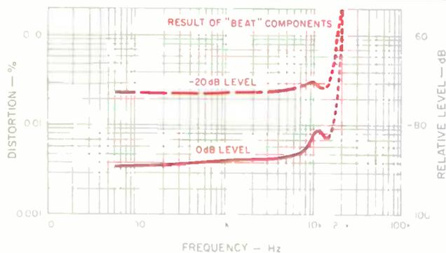
Fig. 3—THD vs. frequency, at two output levels (see text).
