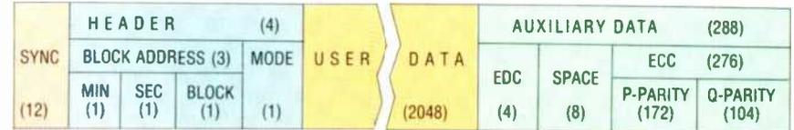
EDC = Error Detection Code, ECC = Error Correction Code
