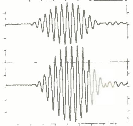
**Fig. 10—Output from 15- and 30-cm/S, 10.8-kHz pulse test, Shure TTR-103 test record. Note the small amount of asymmetry and compression.**
