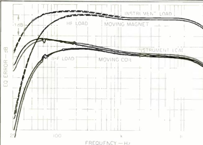
**Fig. 3—RIAA equalization error for 402 preamp's MM and MC inputs, with instrument and IHF loads. Note the low-end roll-off and the expanded scale.**
