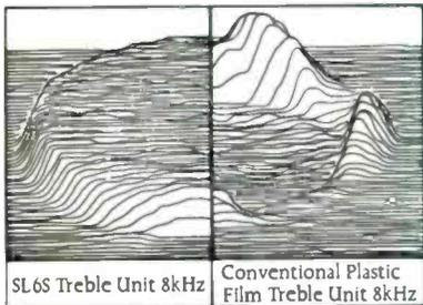
Our computerized laser interferometry mapping system exposes imperfections in driver performance so we can eliminate them.
