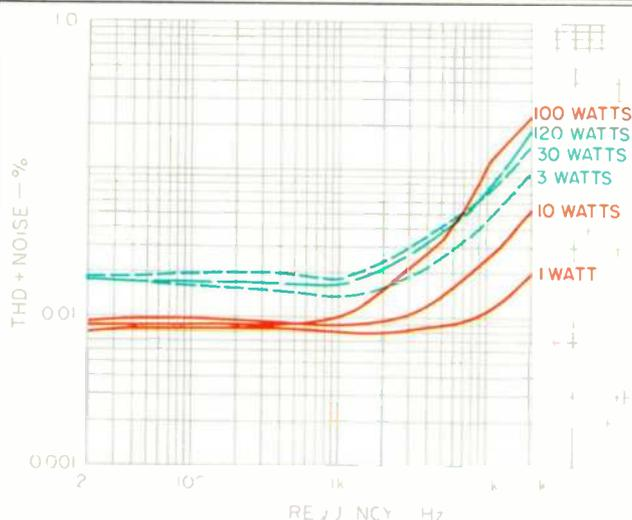
**Fig. 5—THD + N vs. frequency, 702 amplifier, for power levels of 1, 10, and 100 watts into 8 ohms (solid curves) and 3, 30, and 120 watts into 4 ohms (dashed curves).**
