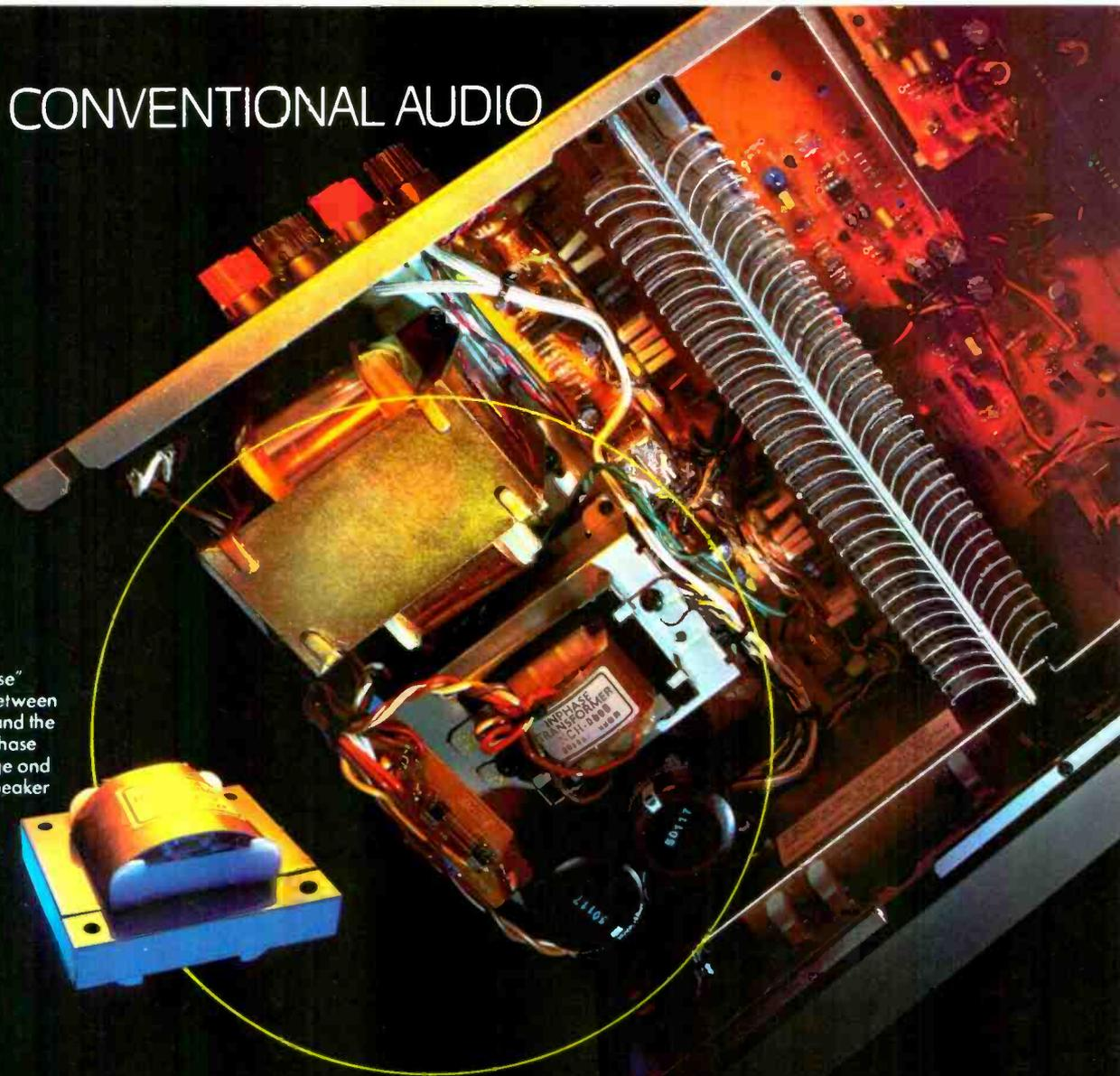
Onkyo's special "In-Phase" Transformer is placed between the power transformer and the capacitors. It prevents phase shift between the voltage and current in the amp-to-speaker signal path that can cause poor stereo imaging and diminished bass response.
