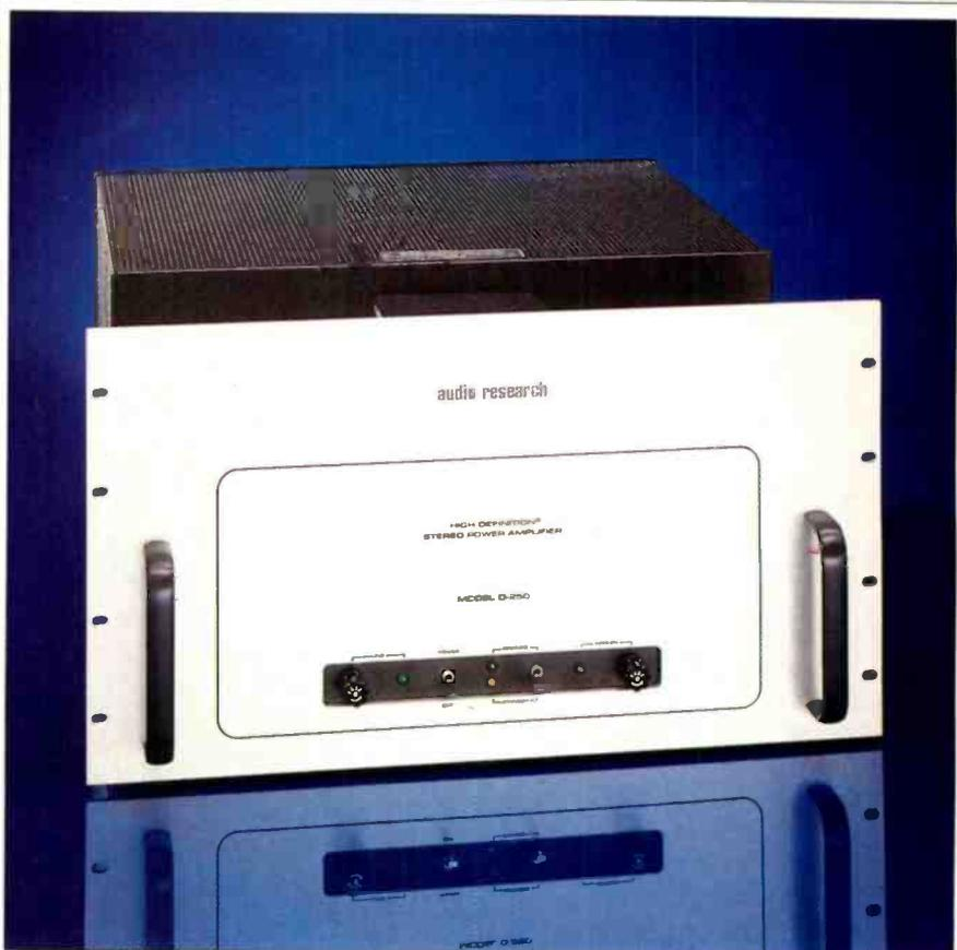
original D-250. The company is now using 6550 output and regulator tubes that are made by Philips (USA) rather than by G.E., and has found that the Philips tubes have a life of up to 2,000 hours in the D-250. The circuit's fusing and key resistors were changed in the Mark II version, and soft-start circuitry is used to largely eliminate any risk of the kind of "meltdown" that would require a service call.
