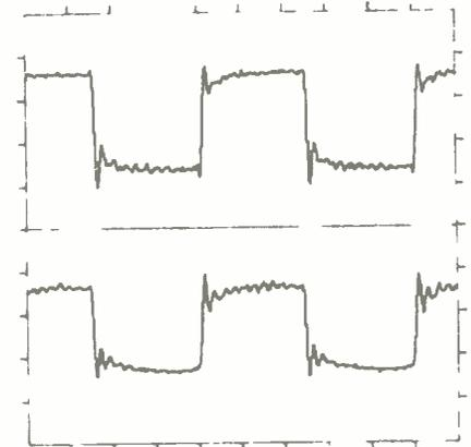
**Fig. 12—Output from 1-kHz square wave, CBS STR-112 test record. Ringing is at 27.8 kHz.**
